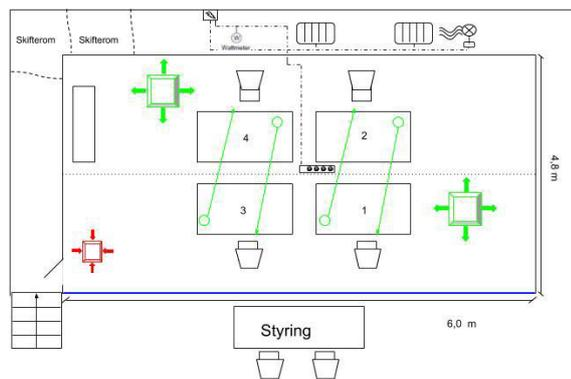
**Figure 1.** Climate chamber setup. Four nozzles placed above desks and two supply air diffusers (green). Extract (red)
