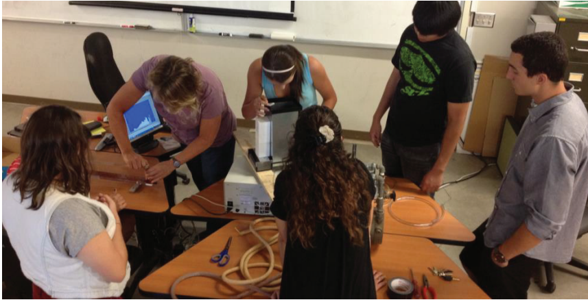
Figure 56: Experiment testing particle removal efficiency of an 3D printed module. The collaborative research team consists of faculty and students from environmental engineering, mechanical engineering, and architecture.
