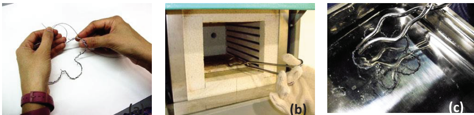
Figure 5. Experimentation with materials with shape memory. (a) Construction of the model, (b) Heat treatment and (c) Tempering.
