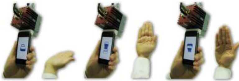
Figure 2.10 Using the pose of the flat hand behind the device (Kratz et al, 2012).
