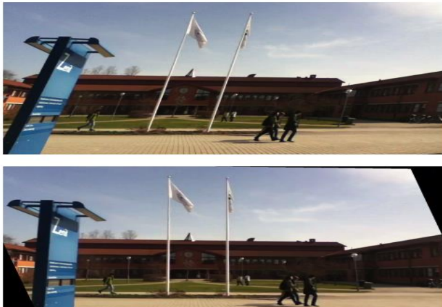
Figure 2.6 Distortion effect and rectified frame using accelerometer and gyroscope (Hanning, et al, 2011)
