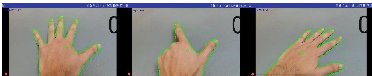
Figure 5.2 Applying convex hull function to detect all bulged out points in the segmented hand area.
