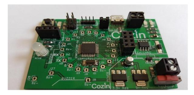
*Figure B.4: A Picture of A fully complete Prototype of Sensor Node (Finished PCB with components)*
