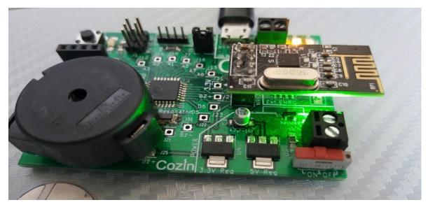
Figure B.5: A Picture of A fully complete Prototype powered with USB cable Note. Image taken with Samsung Galaxy S6 (Smartphone)
