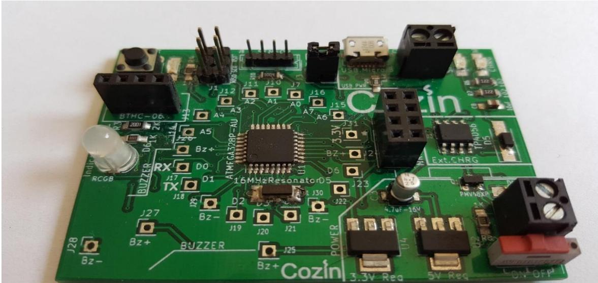
Figure B.4: A Picture of A fully complete Prototype of Sensor Node (Finished PCB with components)
