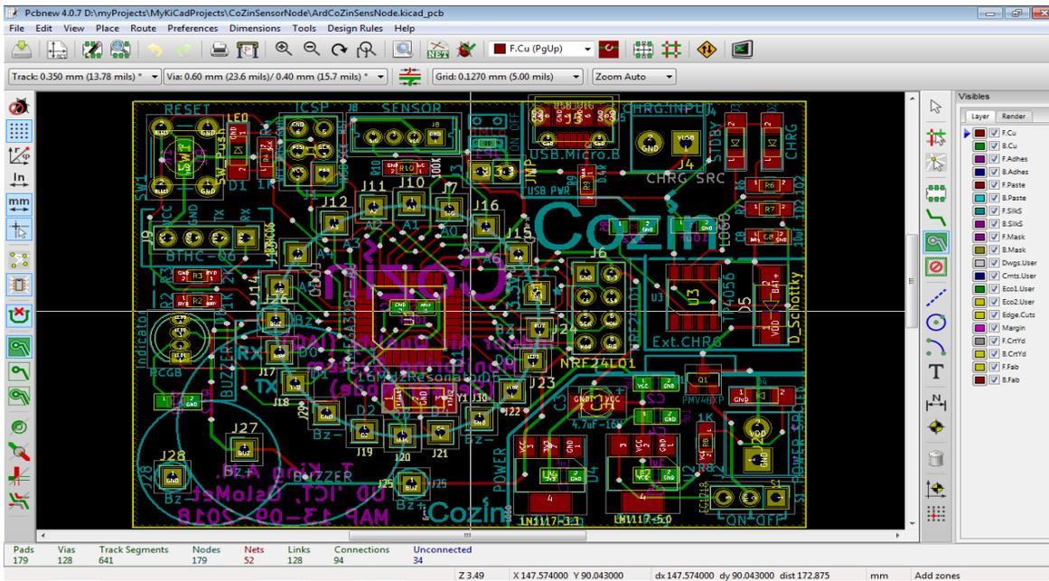
Figure B.2: Screenshot of system prototype Hardware PCB design layout, default view
