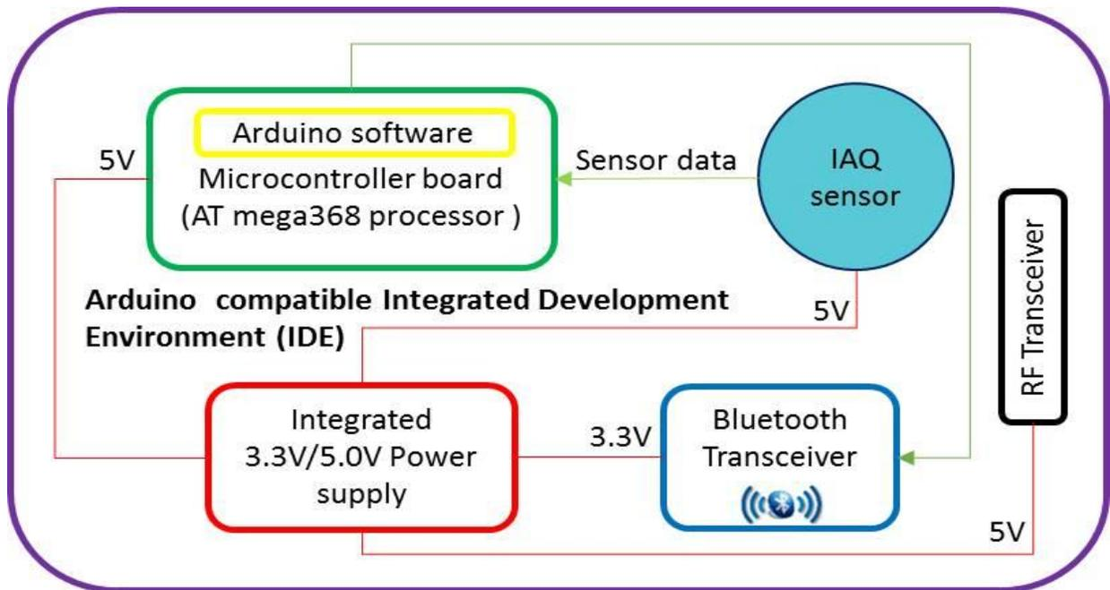
Figure 5.4: Diagram showing all the major components of the Sensor Node
