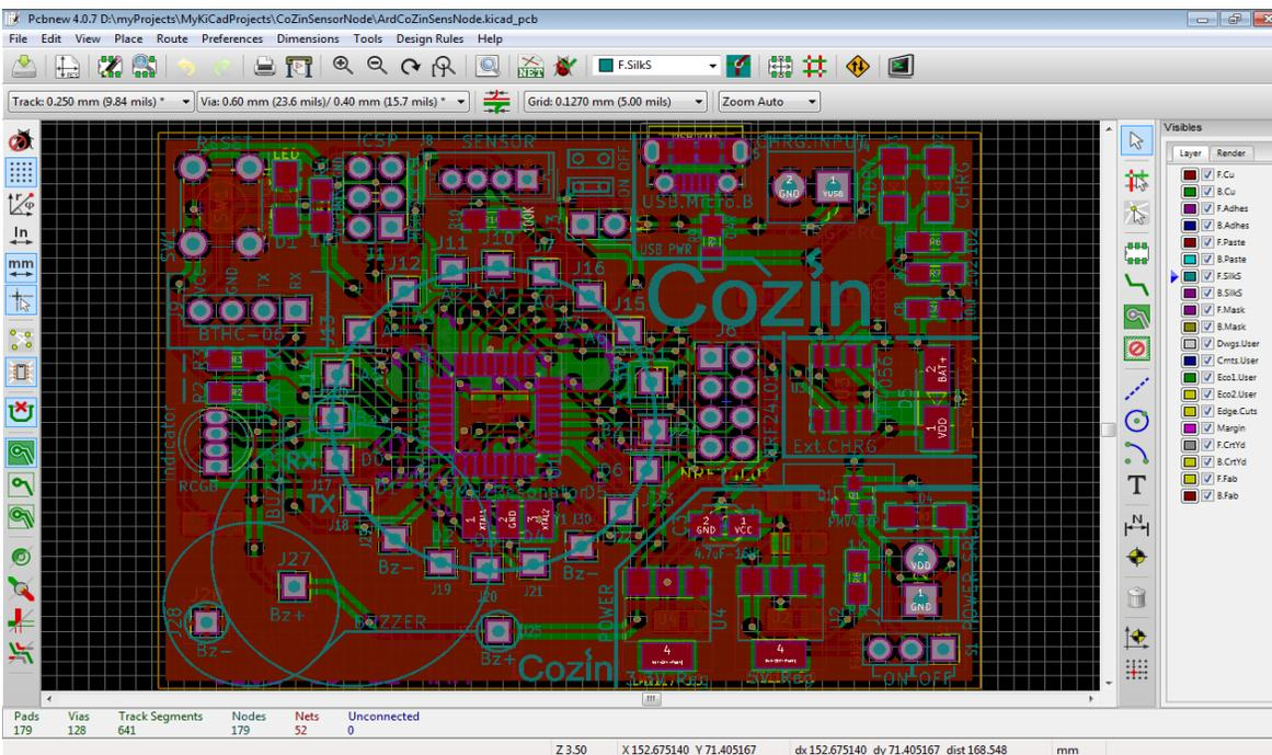
Figure B.3: Screenshot of system prototype Hardware PCB design layout, OpenGL view
