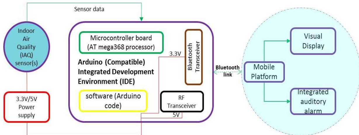
Figure 5.2: System Block Diagram showing all the main features
