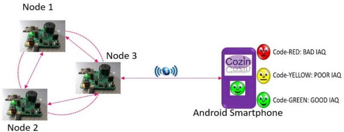
Figure 5.5: Network communication, system function and notification
