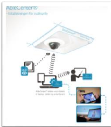
Figure 5 AbleCenter mounted in the ceiling, using wireless communication with smart phones and laptops.
