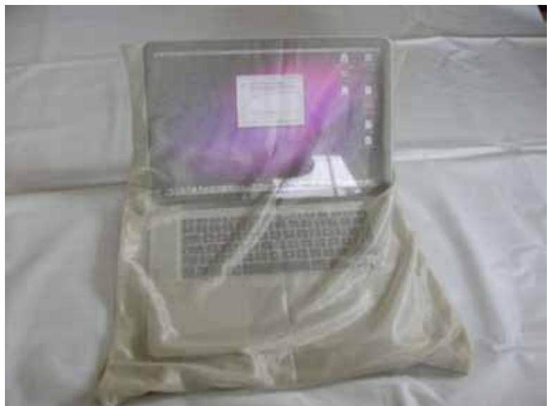
ill. 61: Material demonstration for showing the shielding performance. Internet access becomes limited, but sometimes possible depending on the strenght of the signals
