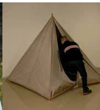
ill. 15: Faraday-tent for experiments and measurements sold by Holland Shielding Systems
