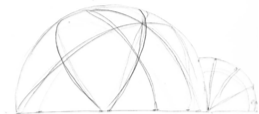
ill. 43: Sketch of dome shaped structure supported by multiple rods of half circles
