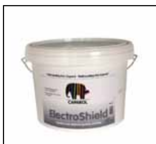
ill. 27: Caparol Electro Shield: Shields frequencies between 200 MHz and 10 GHz. At 36 dB the shielding performance is 99,98 %. This paint contains copper and silver particles.
