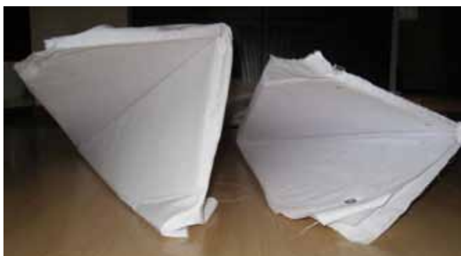
ill. 49: Spring testing: Cellu Float 10 mm height with: (left) 10 mm distance between pieces (right) 15 mm distance between pieces 10 mm provides substantially more spring
