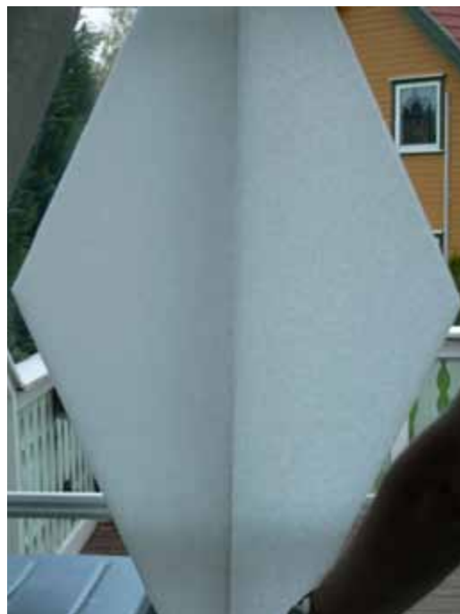
ill. 50: Light transmission testing: left is Ethafoam from Dow and right is Cellu Float
