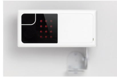
Fig. 2. RoomMate depth sensor deployed in our field trial [3].
