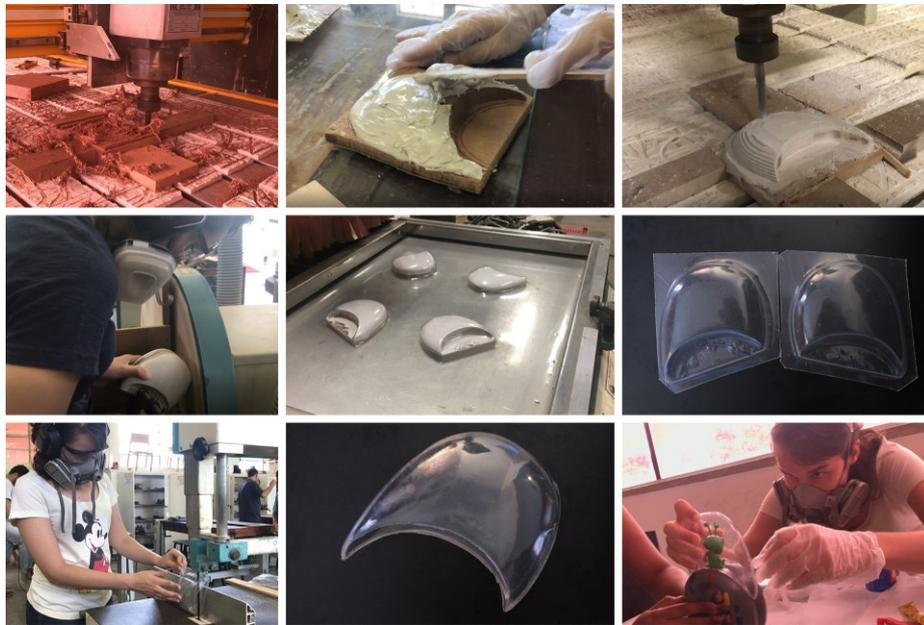
**Fig. 8.** CNC machining and vacuum forming processes used to produce a transparent spaceship cover.
