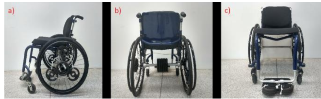
Fig. 1. Added mass on (a) the rear wheels' spokes; (b) on the center of rear wheels' axle; (c) under the foot support.
