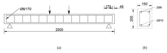
**Figure 2.** Geometry of simulated corroded reinforced concrete (RC) beams investigated by Rodriguez et al. [30] in mm. (a) longitudinal section; (b) cross-section.
