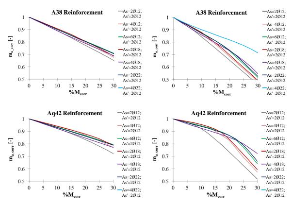
**Figure 11.** Nondimensional ultimate bending moment for existing formed beams: on the left the case of the uniform corrosion, on the right the pitting corrosion.
