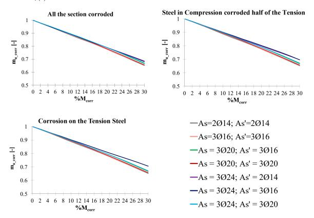
**Figure 6.** Nondimensional ultimate bending moment for different corrosion scenarios—formed Beam, uniform corrosion.
