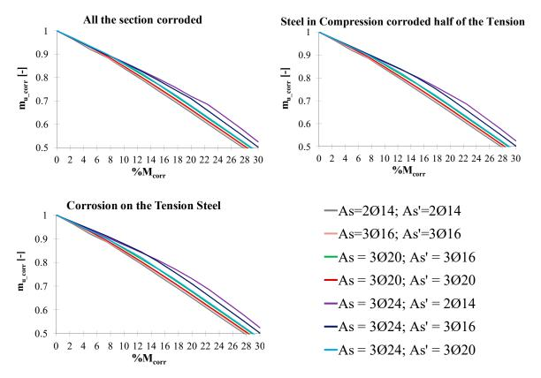
**Figure 8.** Nondimensional ultimate bending moment for different corrosion scenarios—formed Beam, pitting corrosion.
