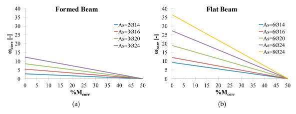
**Figure 5.** Decay of the mechanical reinforcement percentage with the corrosion levels. (a) formed beam; (b) flat beam.
