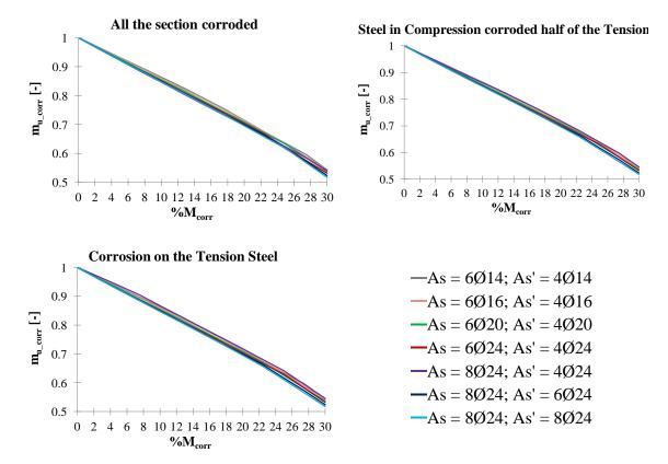
**Figure 9.** Nondimensional ultimate bending moment for different corrosion scenarios—flat beam, pitting corrosion.
