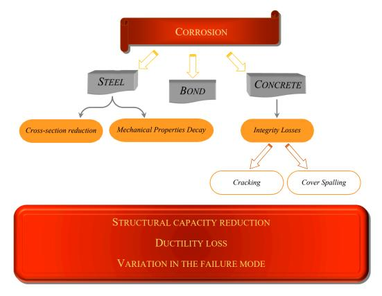
Figure 1. Corrosion influences on the behavior of a structural element.
