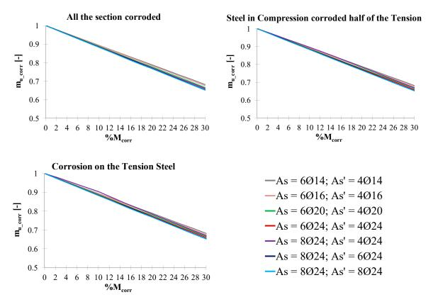
**Figure 7.** Nondimensional ultimate bending moment for different corrosion scenarios—flat Beam, uniform corrosion.
