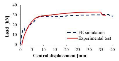
**Figure 4.** Comparison of load displacement curves at mid-span for 2D FE analysis and experimental results of a corroded RC beam no. 115; experimental data from [30].
