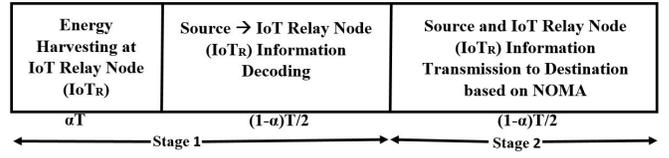
Fig. 2: Proposed system model based on time switching (TS) and NOMA
