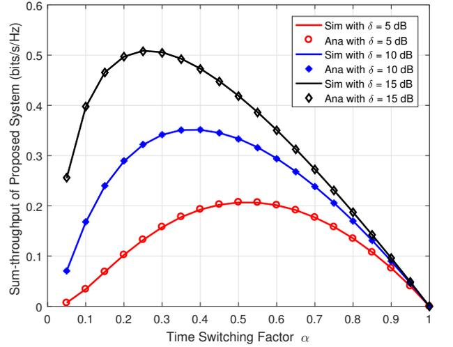
Fig. 6: Sum-throughput of proposed system v/s  $\alpha$  with different  $\delta$
