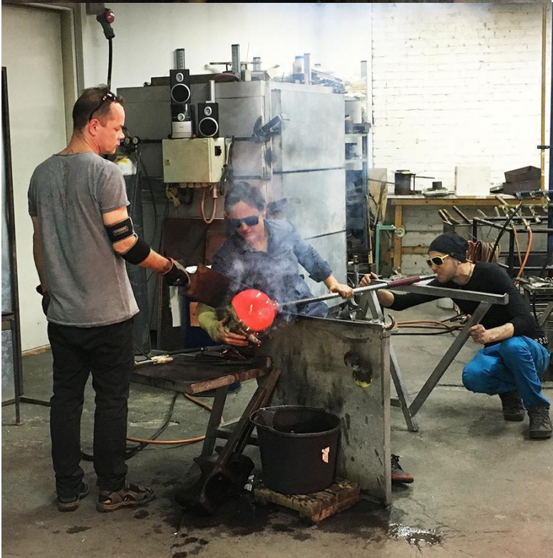
Figure 9 Several craftspeople's collaborative blowing and shaping of the hot glass piece. Photo by the authors.
