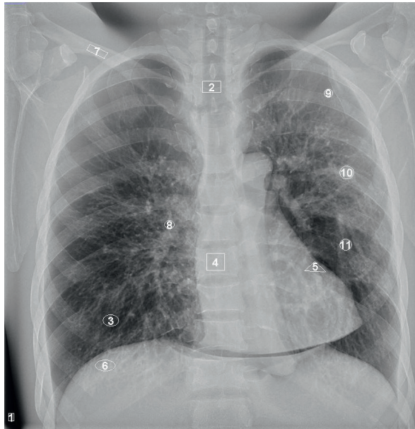
Figure 3: Image of Lungman to demonstrate ROI positions used in the SNR and CNR calculations.
