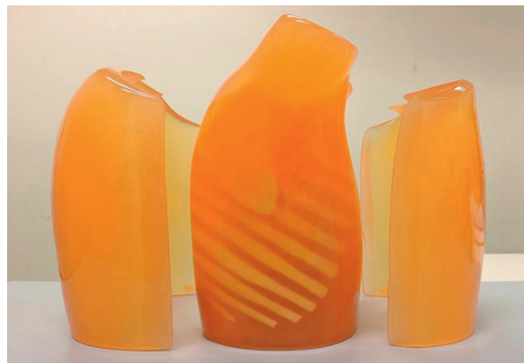
Figure 1: The Lungman multipurpose anthropomorphic adult male chest phantom and 30 mm chest plates.
