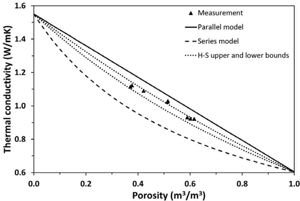
Figure 1– Measured thermal conductivity of plain HCPs submerged in water and analytical bounds [3].
