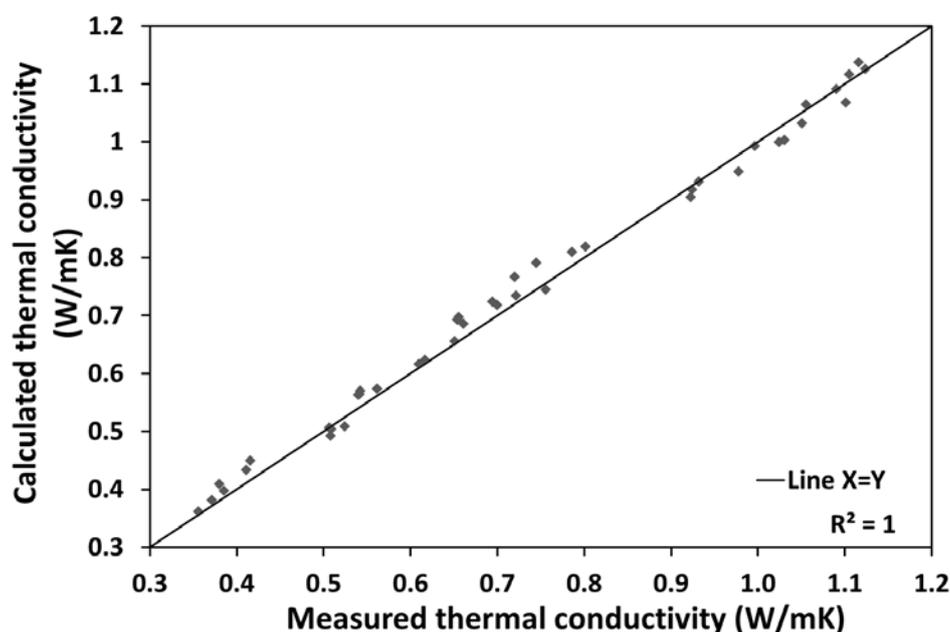
Figure 3 – Comparison of the measured and calculated thermal conductivities [3].
