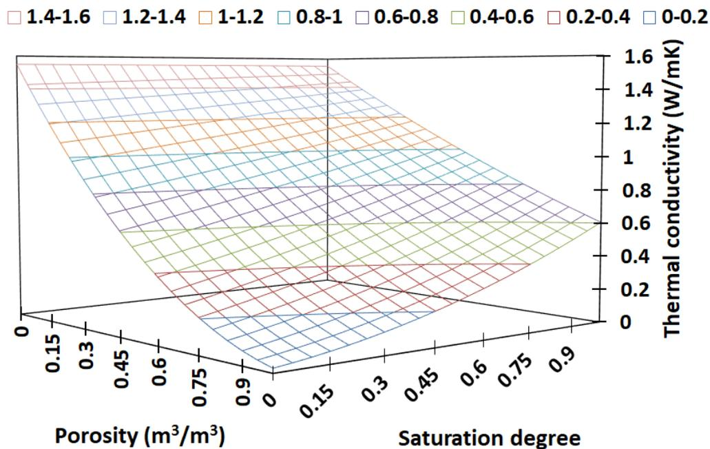
Figure 2 – Thermal conductivity of plain HCPs at different total porosities and saturation degrees calculated from Eq. 9 [3].
