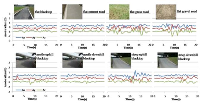
Figure 1. The raw data is generated from the tri-axis accelerometer embedded in a mobile phone that tied on the bike stem. The tri-axis acceleration (Ax, Ay, Az) is measured in time series when bicycling over different terrains.
