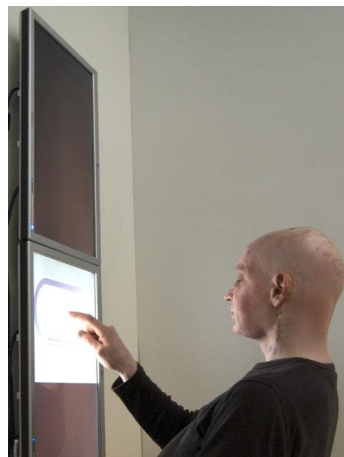
Fig. 1 The interface is positioned at the point of initial touch, in this case at an appropriate height for the user
