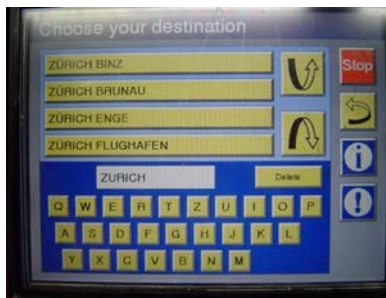
Fig. 9. Destination input with onscreen virtual QWERTY keyboard (from the Swiss Rail Corporation).
