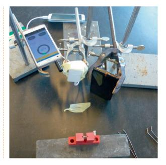
**Figure 3** Setup of the measurement with constant exposure, different distances (15 cm, 30 cm and 45 cm) from the source, to get different dose rates with a <sup>137</sup>Cs source. The image shows the situation with 15 cm.
