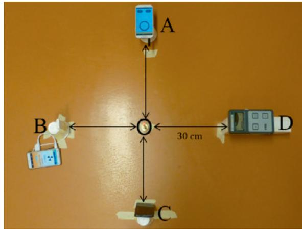
**Figure 3** Setup of the measurement with constant exposure, different distances (15 cm, 30 cm and 45 cm) from the source, to get different dose rates with a  $^{137}\text{Cs}$  source. The image shows the situation with 15 cm.
