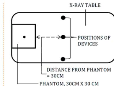
**Figure 1** Setup of the short exposure time measurements
