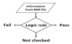
Figure 3: Principle of validation checking
