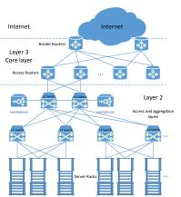
Fig. 1: The architecture of a traditional layered data center.
