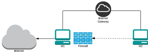
Figure 2: Proposed firewall testing environment.
