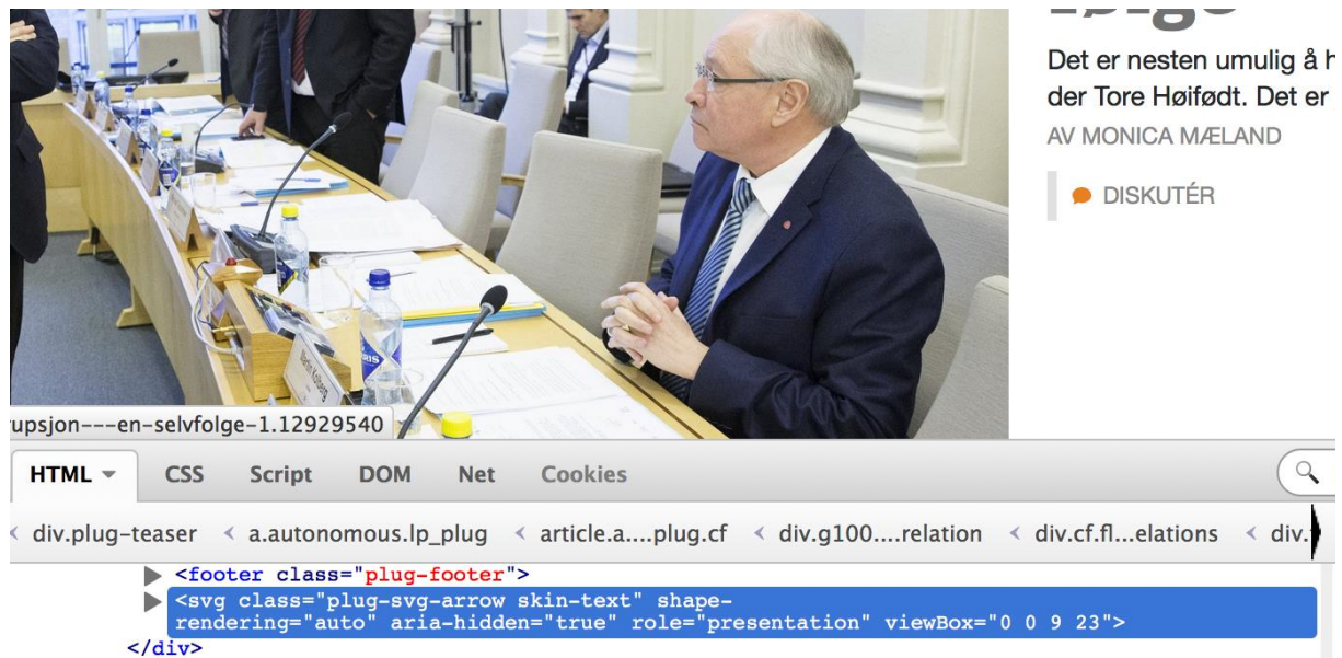
Figure 7.11 The aria-hidden attribute is specified on the icon for Discuss-action link, which allows ATs to skip the icon and move on to the text.
