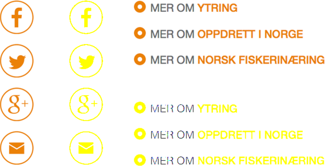
Figure 7.7 Ytring's color scheme provides insufficient contrast between foreground and background for social media buttons and supplemental content
