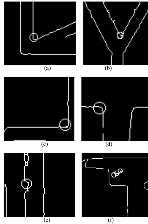
Figure 3. Detected circle, a)-d) non-contamination circle in corners, and e)-f) contamination circles
