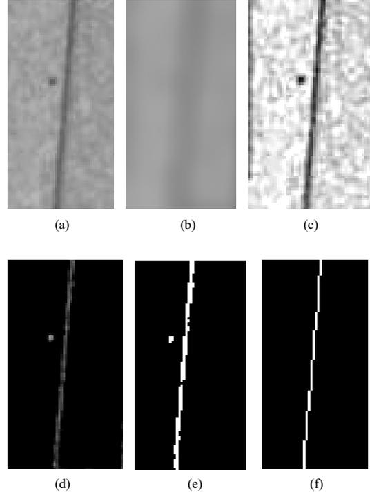
Figure 2. Detected circle and skeleton image; a) gray scale image, b) low-pass, c) high-pass, d) difference image, e) binary image and skeleton, and f) detected circle.
