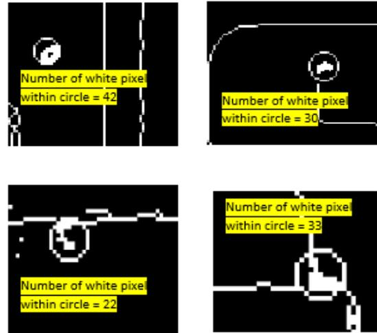
Figure 5. Counting the number of white pixel within a detected circle
