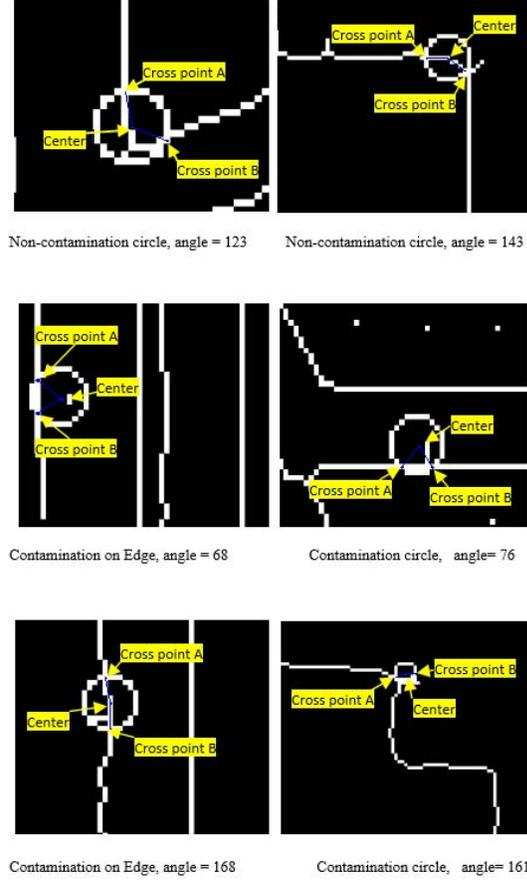
Figure 4. Angle between two cross points and center of circle.
