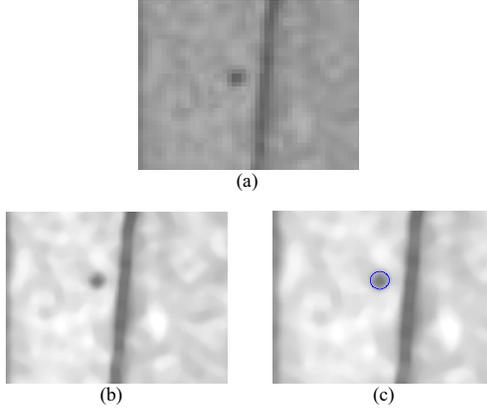
Figure 1. Detected circle in up-sampled image; a) original image, b) up-sampled and median filtered image, and c) detected circle.
