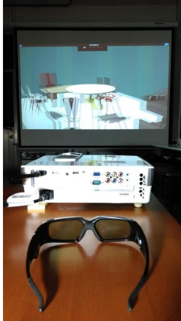
Fig. 3. The 3D projector and the shutter glasses for experiments
