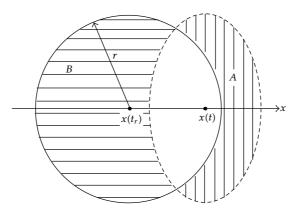
**Figure 4:** The figure shows the difference between a Lorentz contracted sphere (dashed line) centered at the instantaneous current (cur) position of the charge, x(t), and the retarded (ret) sphere (solid line) with the same radius  $r = c(t - t_r)$  centered at the position,  $x(t_r)$ , of the particle at time  $t_r < t$ .
