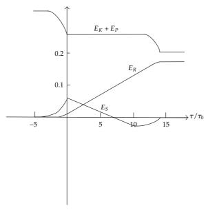
**Figure 8:** Mechanical energy, that is,  $E_K + E_P$ , Schott energy, and radiated energy as functions of proper time. Here  $E_P$  is the potential energy in the force field  $m_0g$  with  $E_P = 0$  for  $X > X_1$ , and  $E_P = m_0g(X_1 - X)$ . Note that  $E_K + E_P + E_S + E_R = \text{constant}$ . All energies are in units of  $m_0$ .
