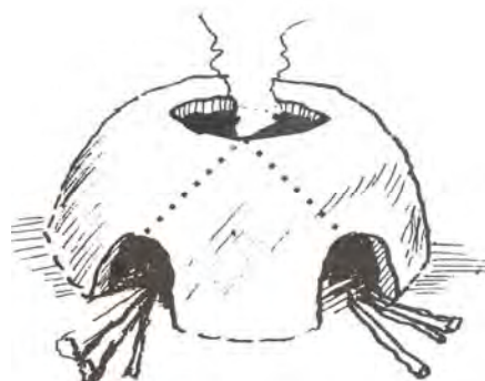
Figure 3.4 Position of the doors in a two-door stove
