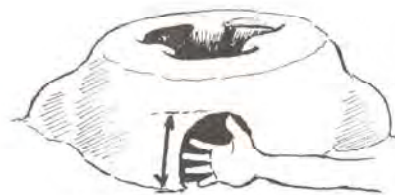
Figure 5.66 The height of the stove door
