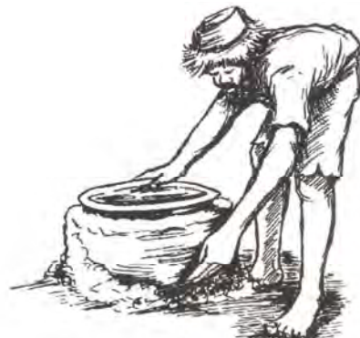
Figure 5.10 Smoothing out the mud
