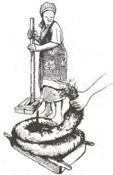
Figure 5.39 Compacting the mud rolls in the mould
