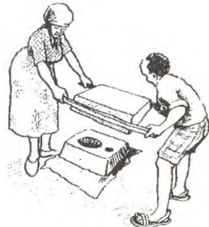
Figure 5.40 Inverting the first mould
