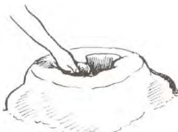
Figure 5.65 Cutting the smoke path
