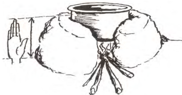
Figure 5.99 The height of the fire chamber
