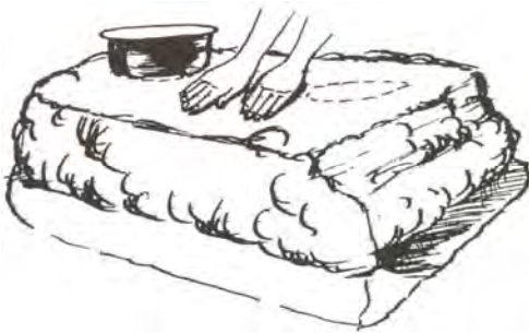
Figure 5.28 Marking the Pot-holes position
