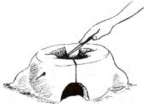
Figure 5.68 Making a smoke vent
