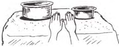
Figure 5.26 Using your palms to space the pot holes
