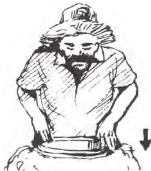
Figure 5.9 Pack the mud to the top of the sufuria
