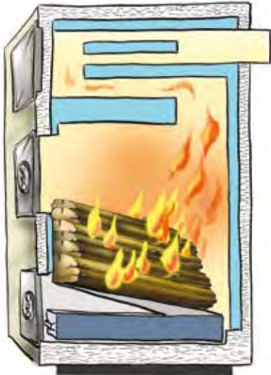
The principle of an over-fire boiler
