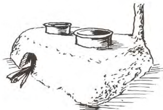
Figure 3.1 Thick walls improve performance of stoves
