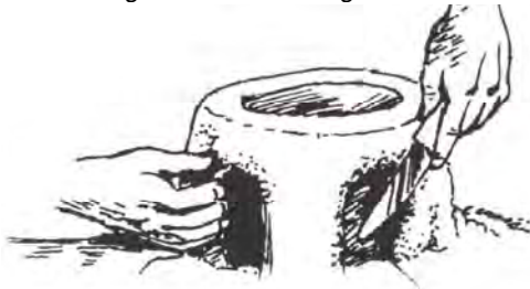
Figure 5.15 Cutting out the doors
