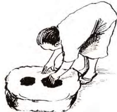
Figure 5.76 Shaping the pot holes
