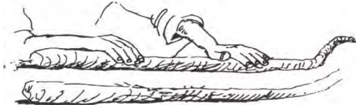
Figure A1.6 Forming long pieces of mud moulds
