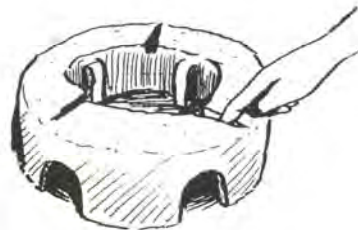
Figure 5.18 Making the smoke outlets
