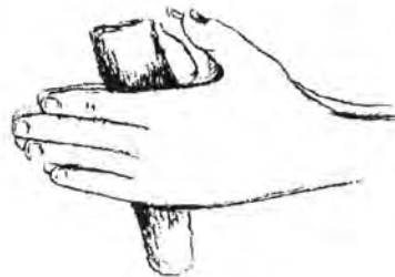
Figure 5.54 Rolling mud to make pot rests
