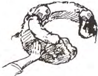
Fixing 5.102 Putting mud around the three stones
