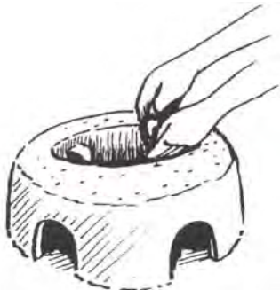
Figure 5.17 Fixing the pot-rests
