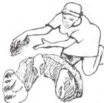
Figure 5.81 Smearing mud around the stones
