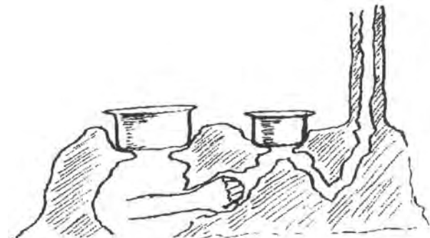
Figure 3.10 The diameter of the connecting channel
