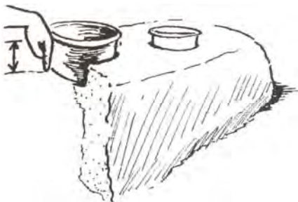
Figure 5.30 Scooping out mud to create fire chambers
