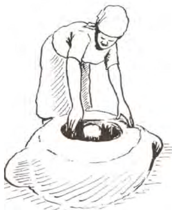
Figure 5.64 Smoothing out the stove
