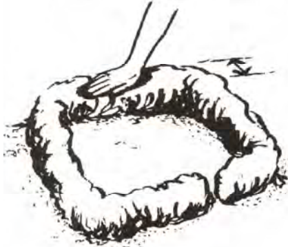
Figure 5.74 Measuring the width of the wall
