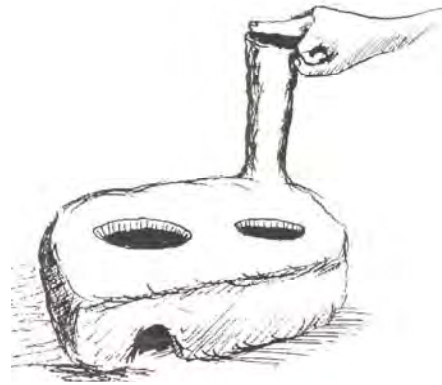
Figure 3.15 Ensuring the chimney diameter is correct
