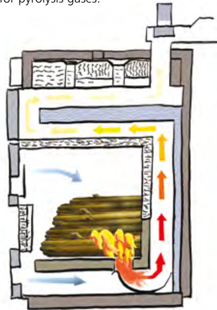
The principle of a down-draught boiler
