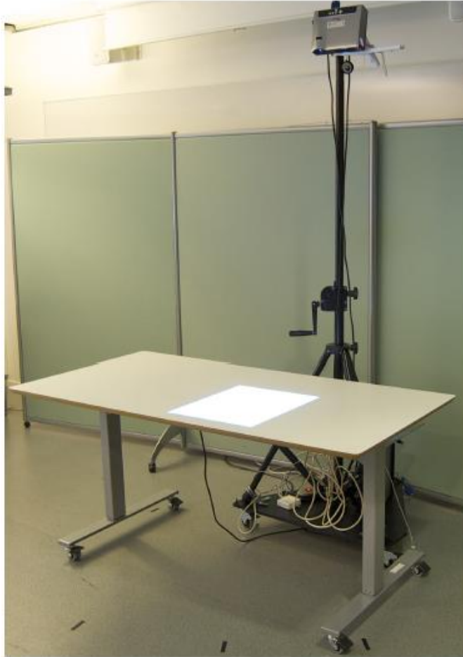
Fig. 1. The prototype comprises a projector mounted on a stand that projects the image onto the surface of a desk. The users interact with the table using mouse, keyboard or handheld devices (iPhone). A more complete prototype could include interaction through hand gestures using touch technology.
