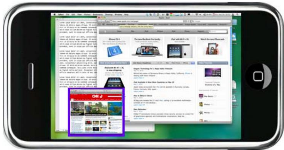
Fig. 2. The surface content shown on the handheld device. The user selects where the selected information (blue border) is to be located when displayed to the other participants.
