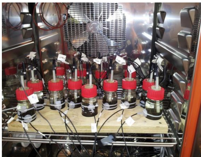
Figure 21: Laboratory setup with microcosms in climate chamber
