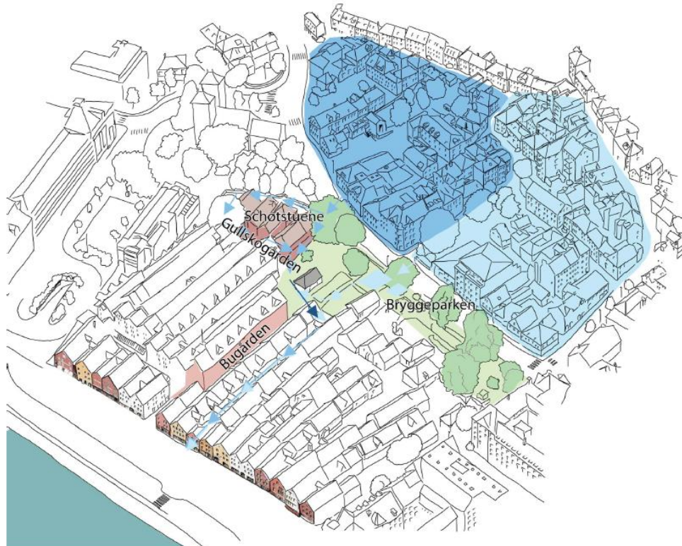
Figure 8: Catchment area behind Bryggen (blue colour) for stormwater collection for potential recharge into the Bryggen area (illustration: Multiconsult AS).
