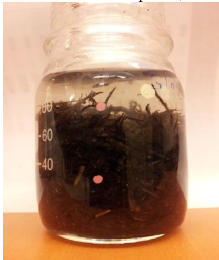
Figure 20: Photo of single microcosm used in laboratory test
