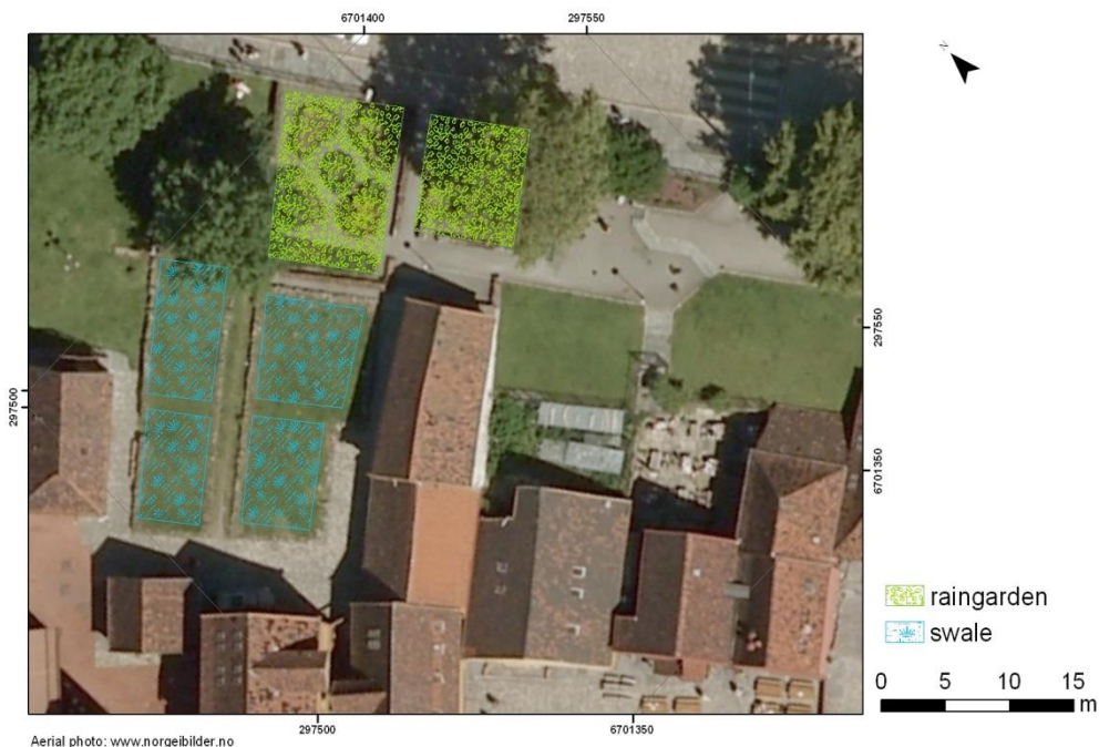
Figure 12: Plan overview of treatment train with rainwater garden, swales and permeable pavement on the lower side of the swales.
