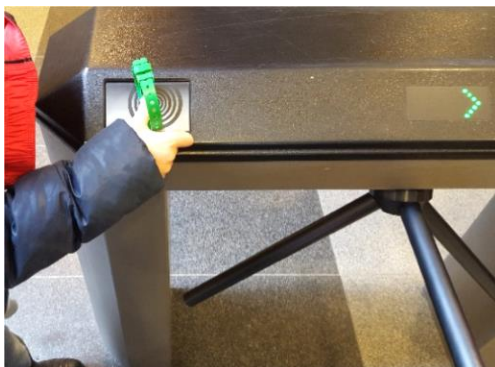
Image 2: A child with the green bracelet letting himself in by tapping it at the RFID-enabled barrier/ Photo: SIFO
