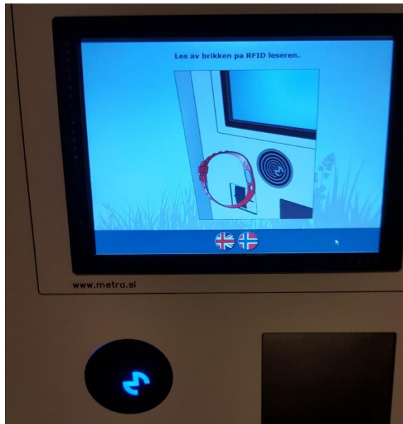
Image 2: Payment machine with touch screen, RFID reader and payment card function / Photos: SIFO
