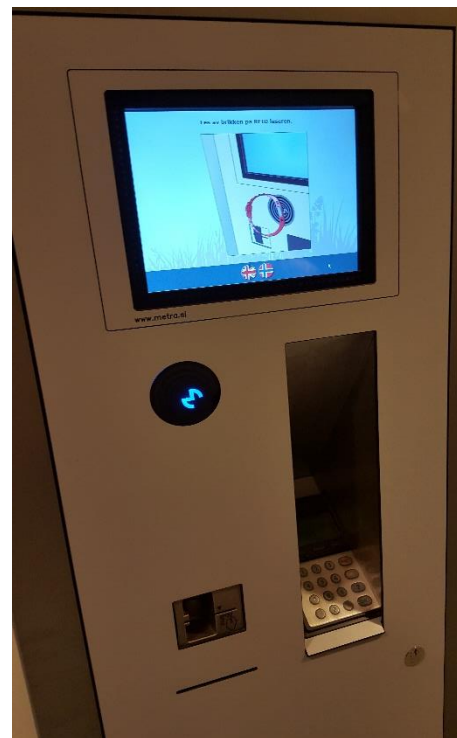
Image 2: Payment machine with touch screen, RFID reader and payment card function / Photos: SIFO
