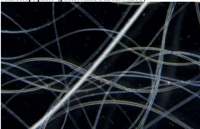
Figure 12 Medullated fibres appear as milky white filled fibres (indicated by red arrow) and are undesirable. Microscope photo (photo: Anne DeBoer/NIBIO)
