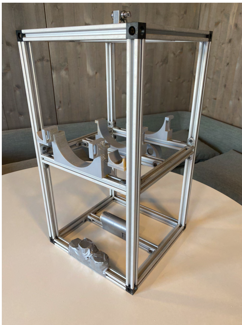
Figure 4.10: Three layer concept with aluminium profiles.
