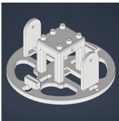
Figure 4.14: Mounting plate for Hall Sensors, Motor(s) and Camera.
