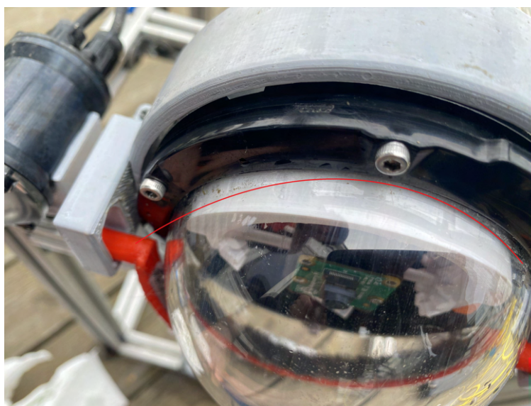
Figure 5.7: Biofouling on the camera dome.
