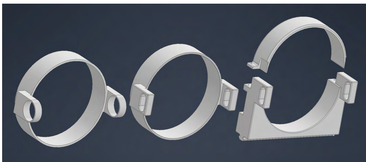
Figure 4.18: 1st (left), 2nd (middle), and 3rd (right) iterations of the outside wiper holder.
