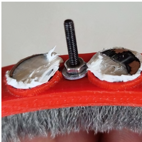
Figure 4.19: Close-up of top of the outer wiper, showing brush attachment method.
