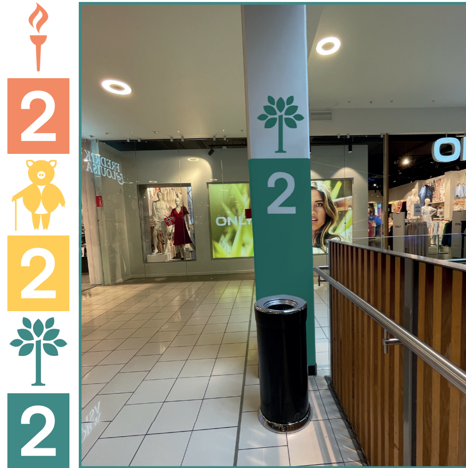
Fig 34 Colored icon and transparent floor number, same on all four sides. Use of positive and negative space. Paint or foil on support beam.
