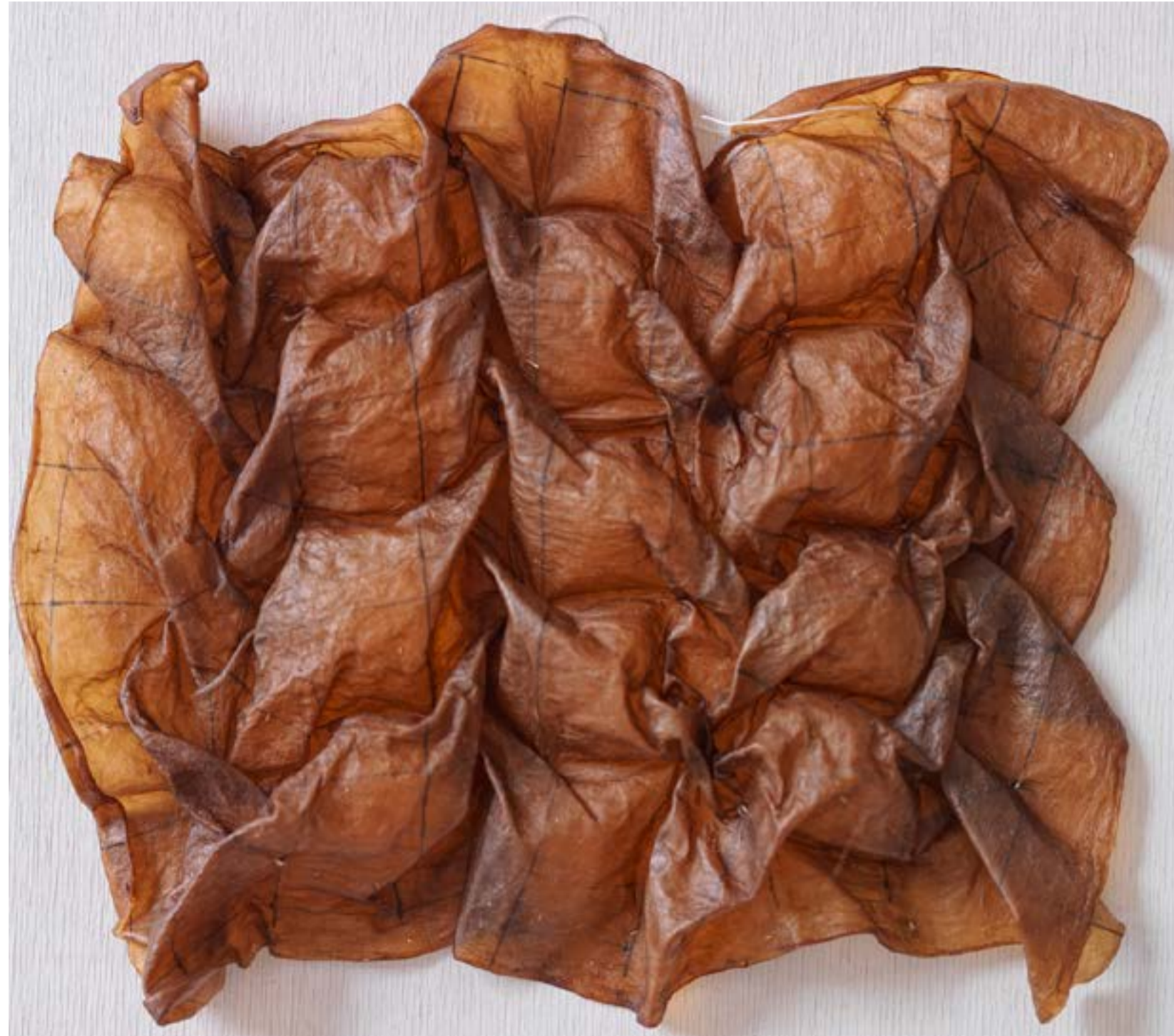
Figure 40: Bacterial cellulose that is over 5 mm and grown on a good culture is flexible and durable when dried. This makes it possible to sew with. It can be joined this way to create patterns.
