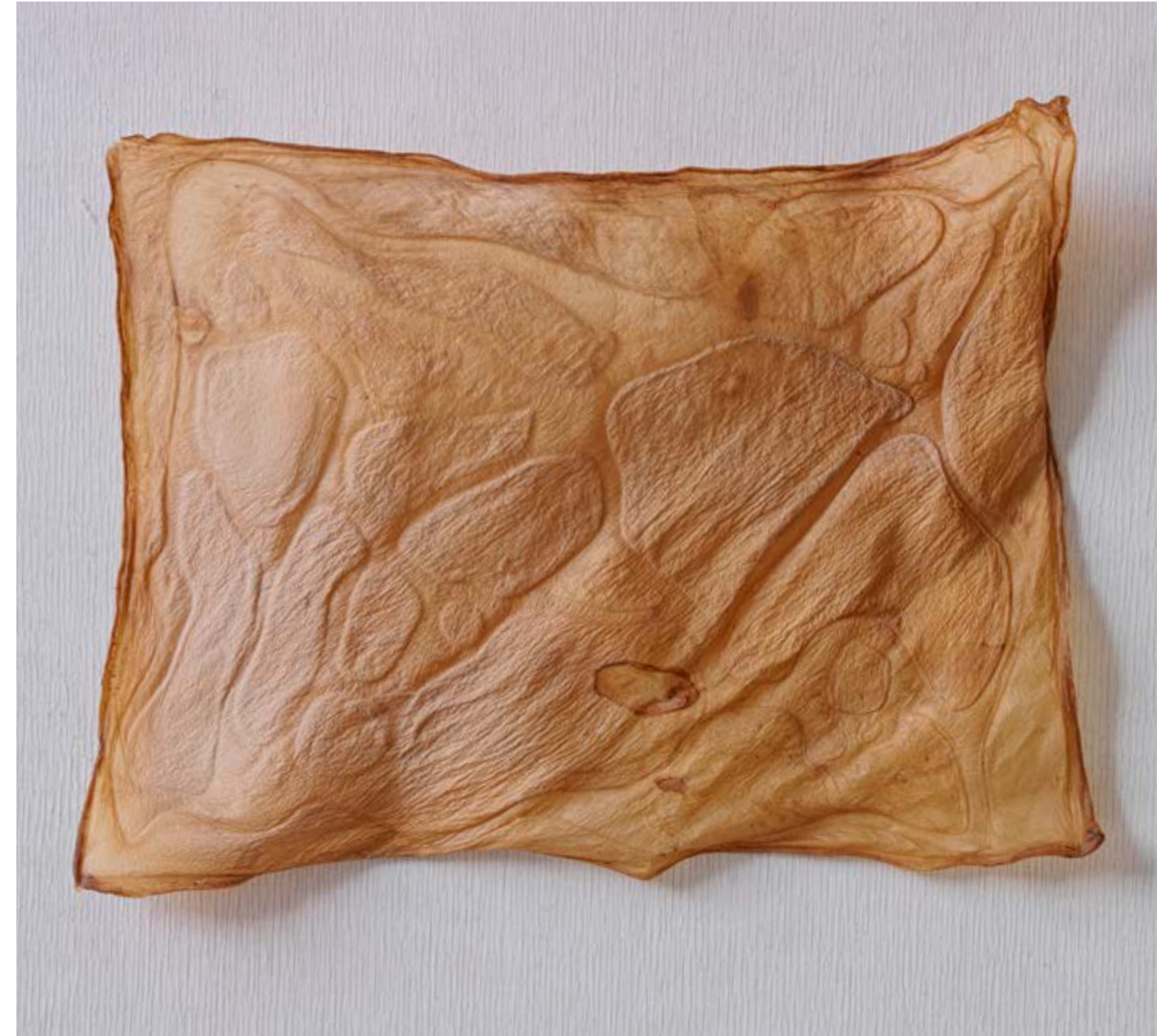
Figure 31: BC patterns. BC dried over 3D-printed PLA, the pattern is drawn in fusion360, and is ment to mimic bacterial growth
