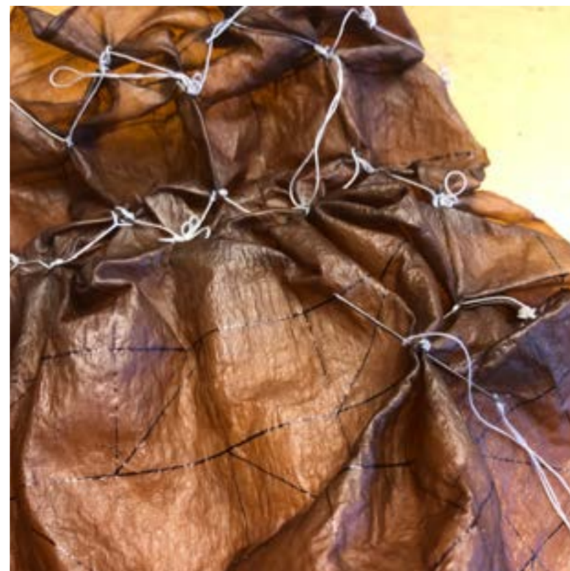
Figure 12: sewing BC, thickness makes it harder to sew into that regular fabric
