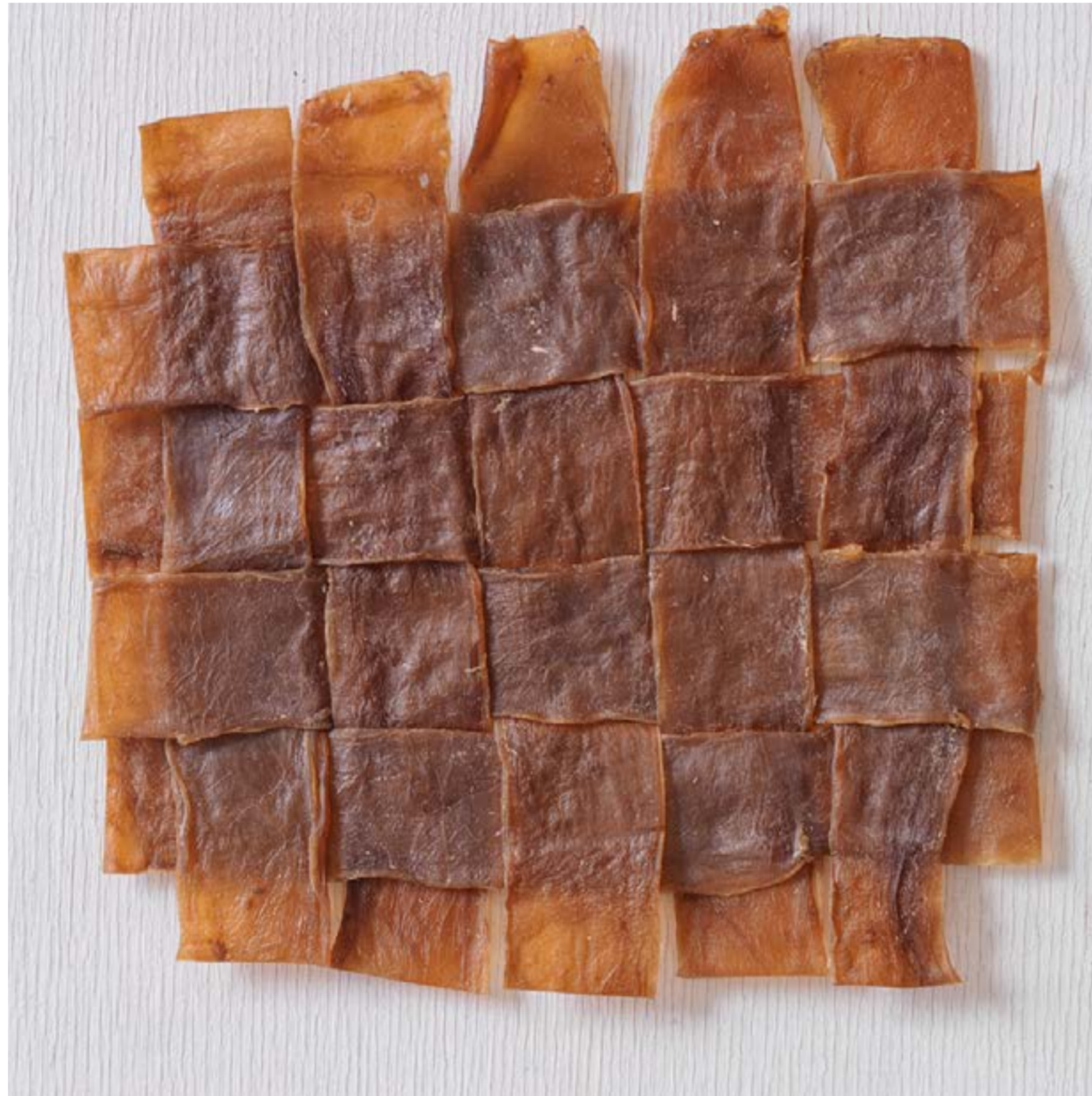
Figure 36: Cutting BC. BC cut when wet and joined by using basket weave technique
