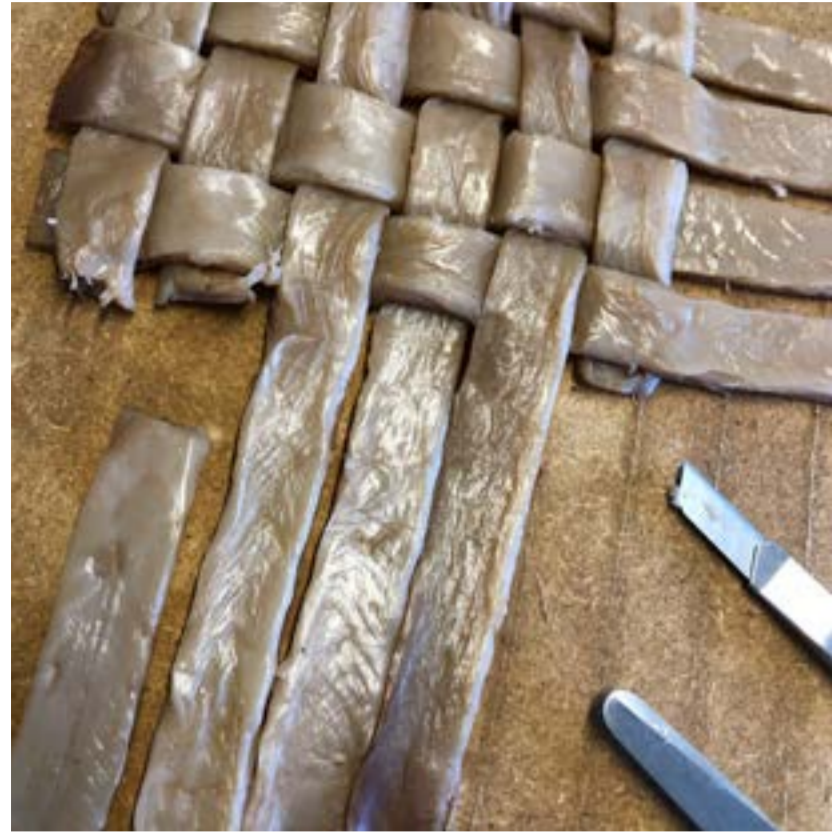
Figure 9: Cutting BC, and joining using basket weave technique
