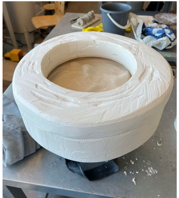
Image depicting a plastermould of the first iteration of the Atlas platter. The mould is used for both slipcasting and presspiling.
