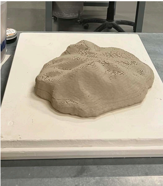
Image depicting a clay printed object that would later, after the initial bisque firing, be used as a hump mould by pressing and so forming a slab of clay over this form.
