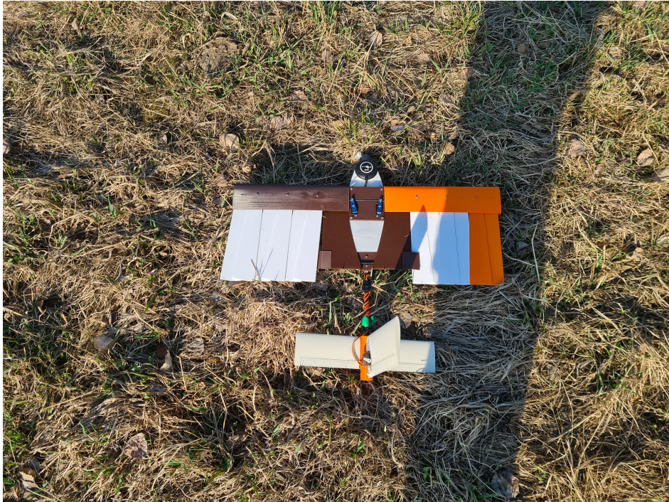
Figure 4.9: Test flight four - attempt one crash
