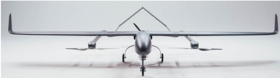
(b) Hybrid VTOL fixed-wing, picture from [4]
