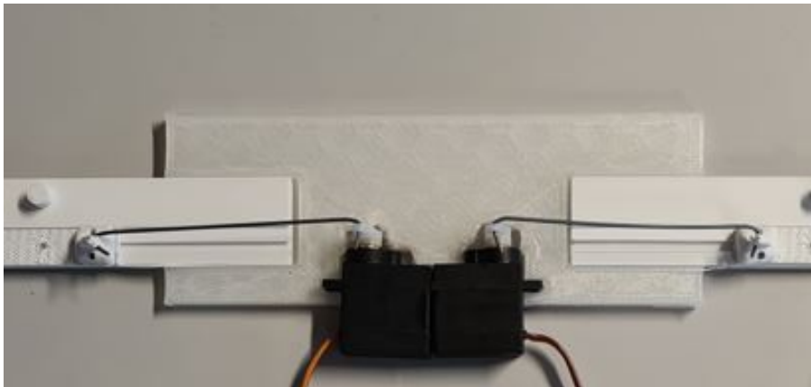
(b) Servos and sliding base installed on wing platform
