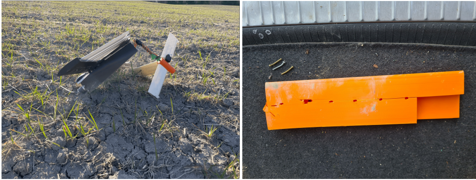
(a) Test flight four attempt three crash (b) Damage from test flight four attempt three crash
