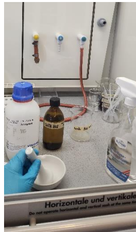
Fig.3. 11. Agate mortar cleaning in the fume hood with diluted HCl acid and isopropanol.
