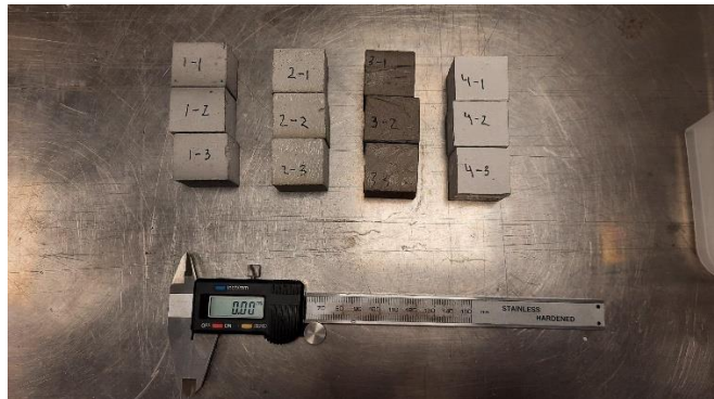
Figure 46 All Tile Adhesive Specimens Finalized and Identified – Ready for Sorption Experiment
