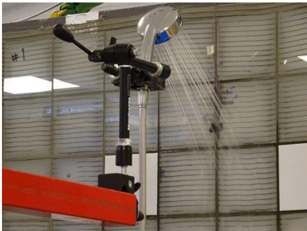
Figure 63 Shower Water Exposure Target Area Impacting the EUT
