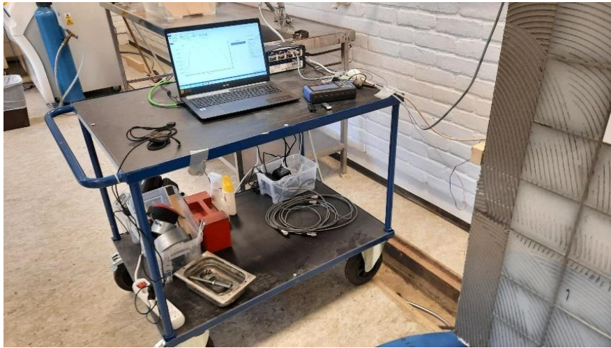
Figure 44 Data Acquisition Hub Showing all Critical Data Acquisition Equipment
