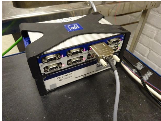
Figure 51 Quantum X used for Weight Logging Signal Processing
