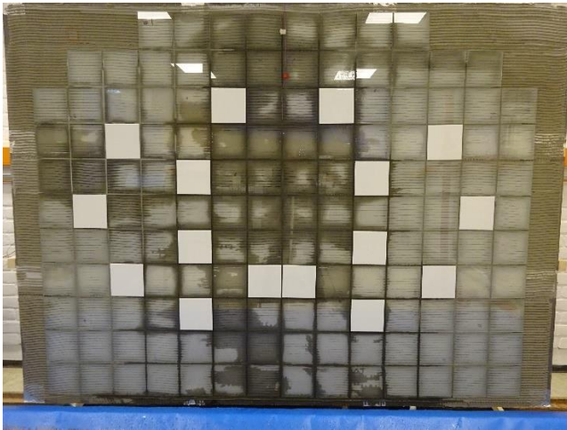
Figure 70 EUT #1 after a Total of 424 min of Water Exposure incl 96 hours of Soaking
