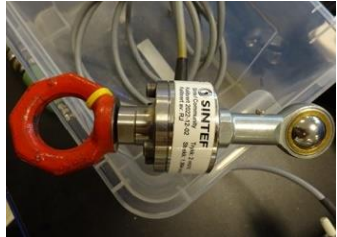
Figure 50 Load Cell with Eyebolt for Measuring the Weight of the Wall
