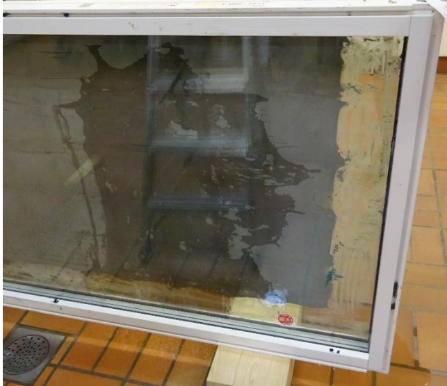
Figure 16 Water Exposure after 8 min – Without Grout between the Tiles
