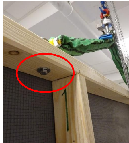
Figure 23 Wall Hoisting Assembly Bolt for Mounting Wall to Ceiling
