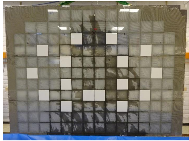
Figure 103 Wall #4 Visible Moisture Content after 288 min Water Exposure
