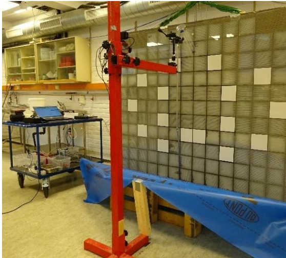
Figure 39 Shower- and GoPro Stand in front of EUT#1
