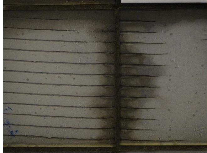
Figure 98 Moisture in Tile Adhesive Showing Saturation (RH = 100 %) in Dark Grey and RH < 100 % due to Diffusion in Light Grey
