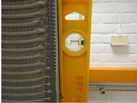
Figure 35 Levelling of x- and y-Axis Using the Hultafors Level
