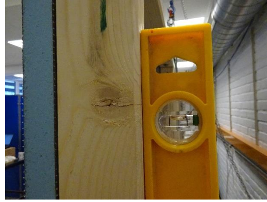
Figure 36 Levelling of the z-Axis Using the Hultafors Level
