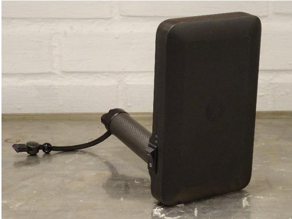
Figure 58 InviSense Scanner used for RH-Sensor Readings
