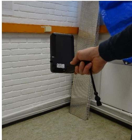
Figure 60 InviSense Calibration, Making Sure no Obstacle is within 1 Meter in all Directions
