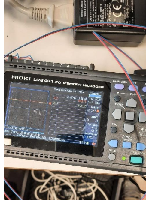
Figure 56 HIOKI Unit during Temperature Calibration
