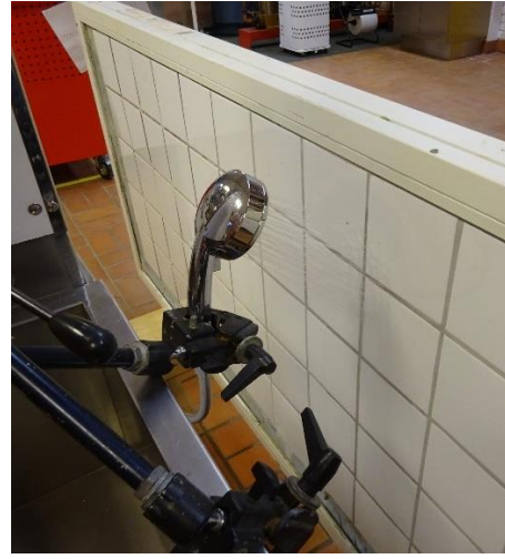
Figure 15 Prototype Water Exposure Setup with Grout between Tiles
