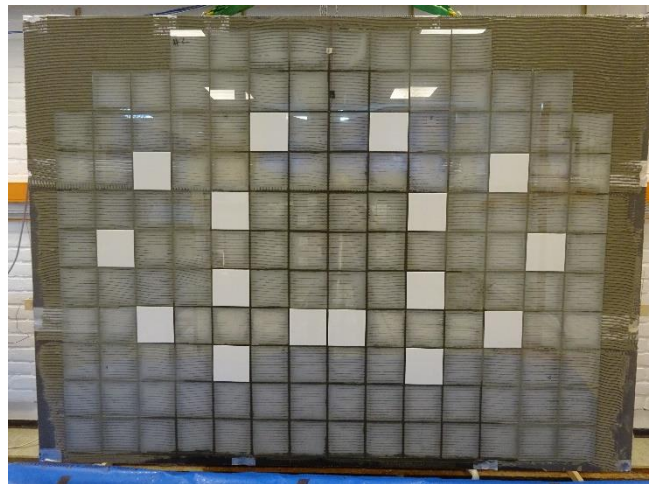
Figure 76 EUT #2 after 96 min of Water Exposure Showing Wet Grout
