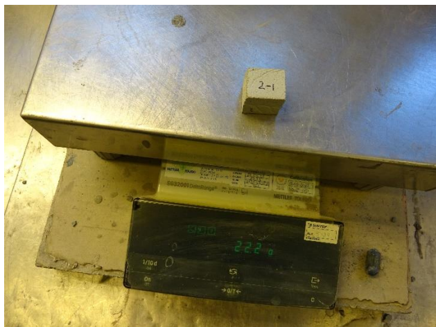
Figure 48 Weighing Tile Adhesive Specimen 2-1
