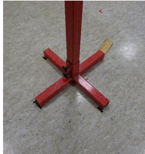
Figure 40 Steel Stand Positioning showing Floor Tape Markers for Repetitive Measurements
