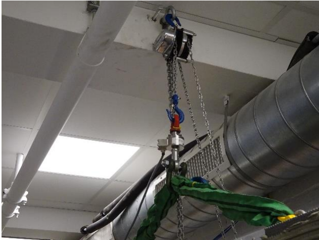
Figure 49 EUT Hanging from the Ceiling in a Load Cell and Pulley Setup
