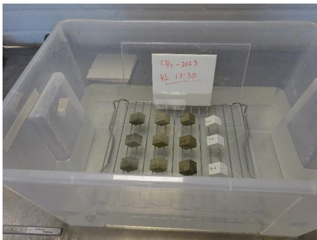
Figure 47 All Tile Adhesive Specimens Submerged in Water
