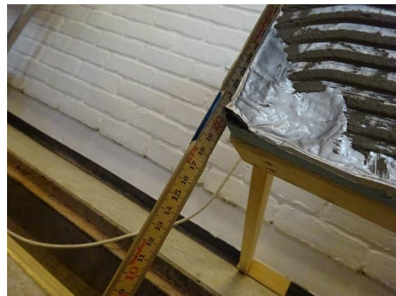
Figure 38 Correct EUT Positioning Elevated 200 mm from the Floor
