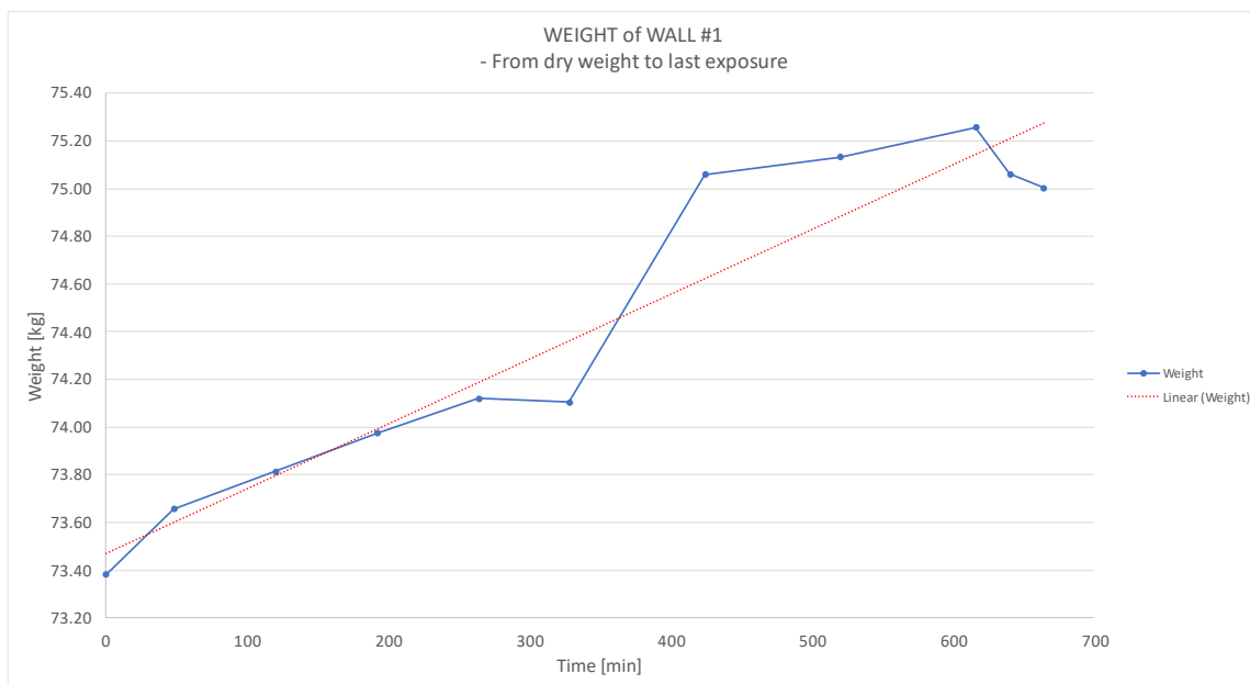
Figure 74 Weight Data of Wall #1 - Daily Post Water Exposure Weight Measurements
