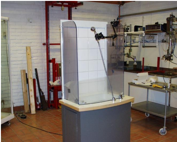
Figure 5 Grout Experiment Setup with Shower Head Aimed at the Tiled Wall
