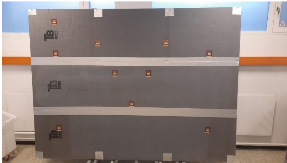
Figure 24 Overview of the RH-Sensor Locations Attached to the Based Wall
