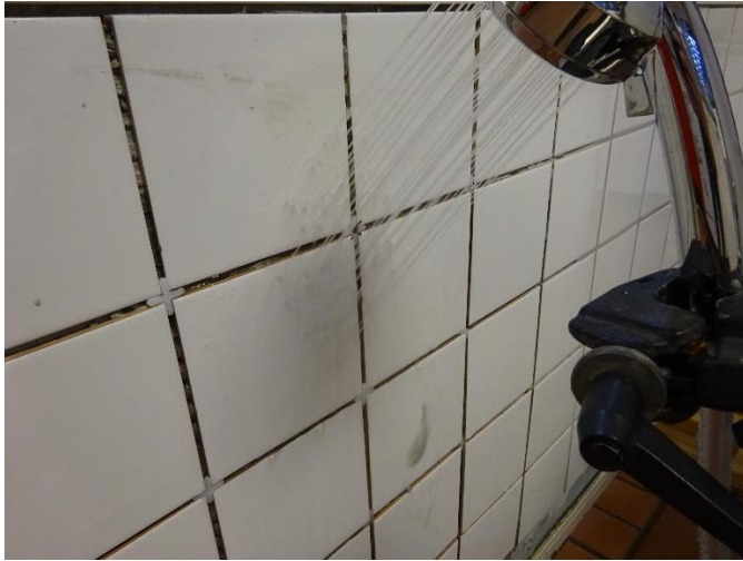
Figure 14 Prototype Water Exposure Setup without Grout between Tiles
