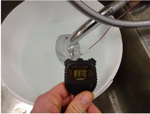
Figure 65 Flow Rate Calibration Timing of 30 Seconds
