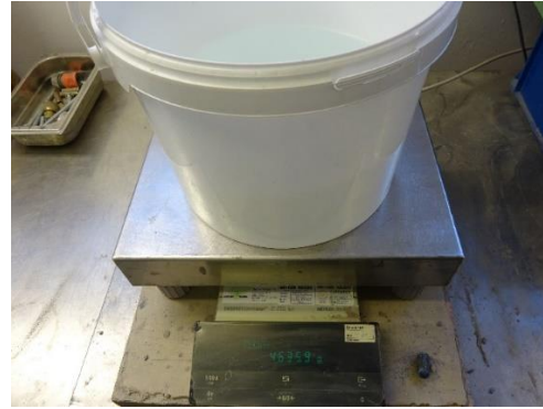
Figure 66 Water Weight of 4 636 Grams after 30 Seconds of Water Flow
