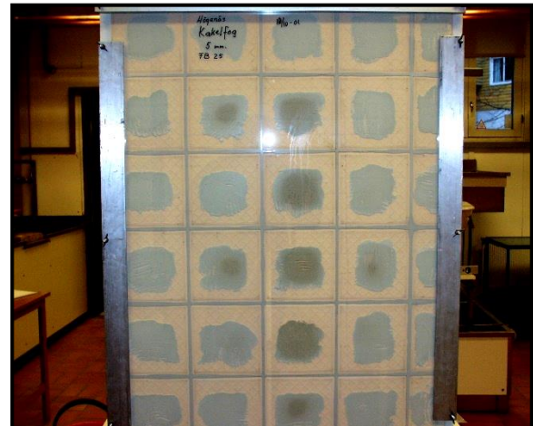
Figure 6 Tiled Wall Seen from the Rear Showing Tiles and Tile Adhesive.
