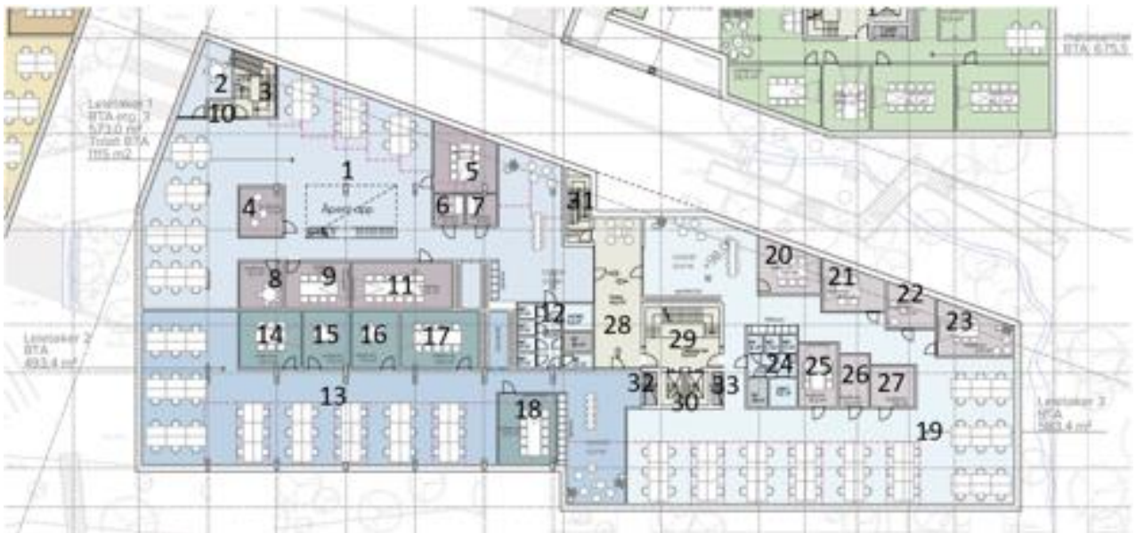
Figure 26. Room number used in calculations of air volume. The project with developing Bøkkerveien 1-3 is in an early phase and changes will occur to the project and floorplan. Figure with permission from Høegh Eiendom AS. [33]
