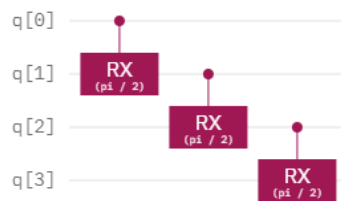
Figure 4.7: A quantum circuit containing the ladder scheme with C-RX instead of CNOT
