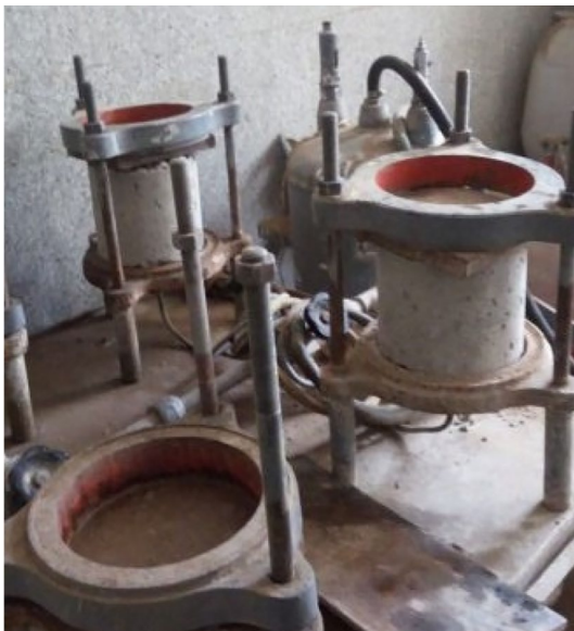
Fig. 6 Semi-cylindrical specimens in water permeability test
