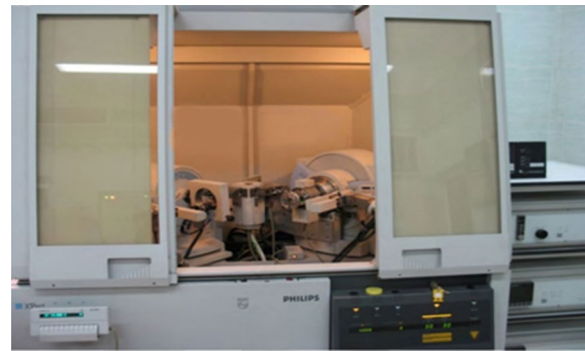
Fig. 4 X'pert diffractometer conducting XRD test
