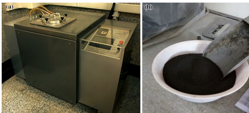
Fig. 3 Sludge burning process: a electric sludge burning incinerator and b obtained sewage sludge ash (SSA)
