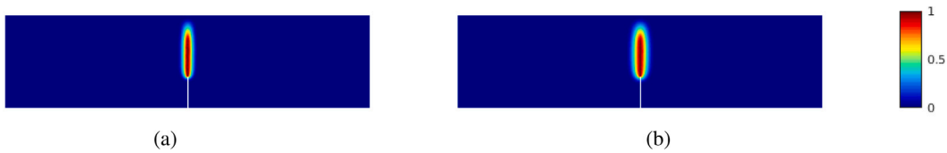
Fig. 7. Damage evolution under different length scales. (a) CMOD = 0.3 mm, l_o = 5 mm, (b) CMOD = 0.3 mm, l_o = 7 mm.
