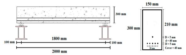
Figure 1. Beam dimensions and cross-section details.
