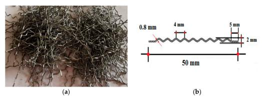
**Figure 2.** The appearance of corrugated and hooked-end steel fibers: (**a**) Clump of the steel fibersand (**b**) Steel fiber size.
