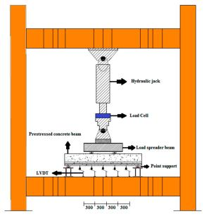
Figure 9. Schematic of the four-point flexural test setup.
