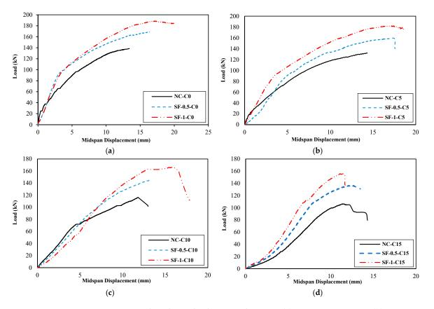
**Figure 11.** Load–midspan displacement diagrams: (**a**) Group A specimens, (**b**) Group B specimens, (**c**) Group C specimens, and (**d**) Group D specimens.
