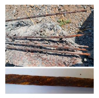
Figure 6. Corroded prestressing wires.
