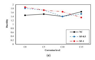
**Figure 16.** Changes in the studied characteristics with increasing corrosion levels: (**a**) bearing capacity, (**b**) midspan displacement, (**c**) energy absorption, (**d**) effective hardness, and (**e**) ductility.
