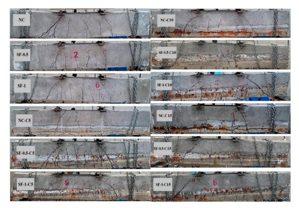
Figure 17. Failure mode and crack pattern of beams.
