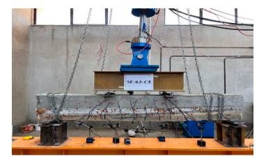
Figure 8. Four-point bending test setup.
