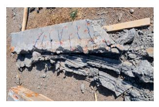
Figure 7. Destruction of specimens and removal of prestressing wires.
