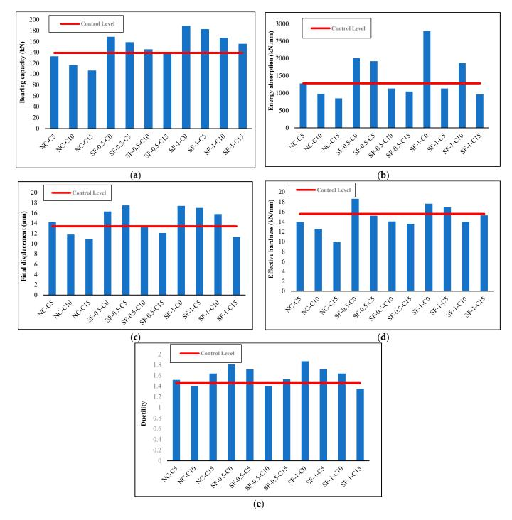
**Figure 14.** Comparative diagram of the change in (**a**) bearing capacity, (**b**) energy absorption, (**c**) final displacement, (**d**) effective hardness, and (**e**) ductility of the beams compared to the control specimen.
