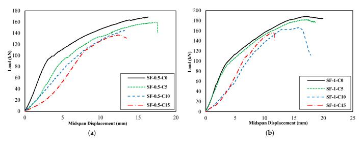
**Figure 13.** Load–midspan displacement diagrams: (**a**) specimens with a 0.5% volume fraction, (**b**) specimens with a 1.0% volume fraction.
