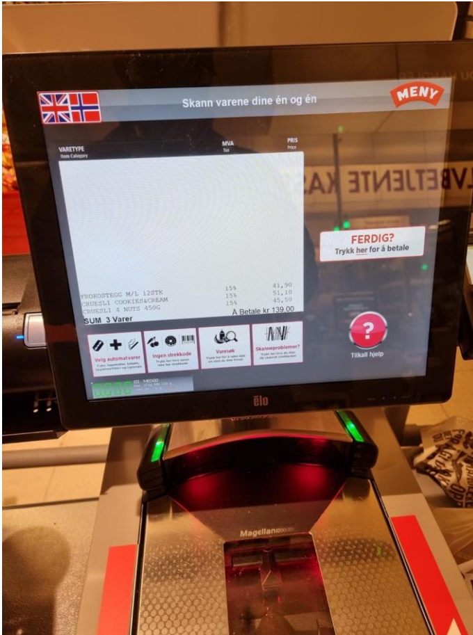
Figure 15 Self-checkout in store, display is reflective
