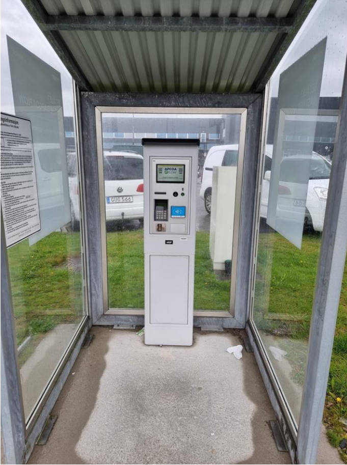
Figure 12 Parking ticket machine, with a special enclosure to protect it from the elements, and reduce reflection from the sun on the display
