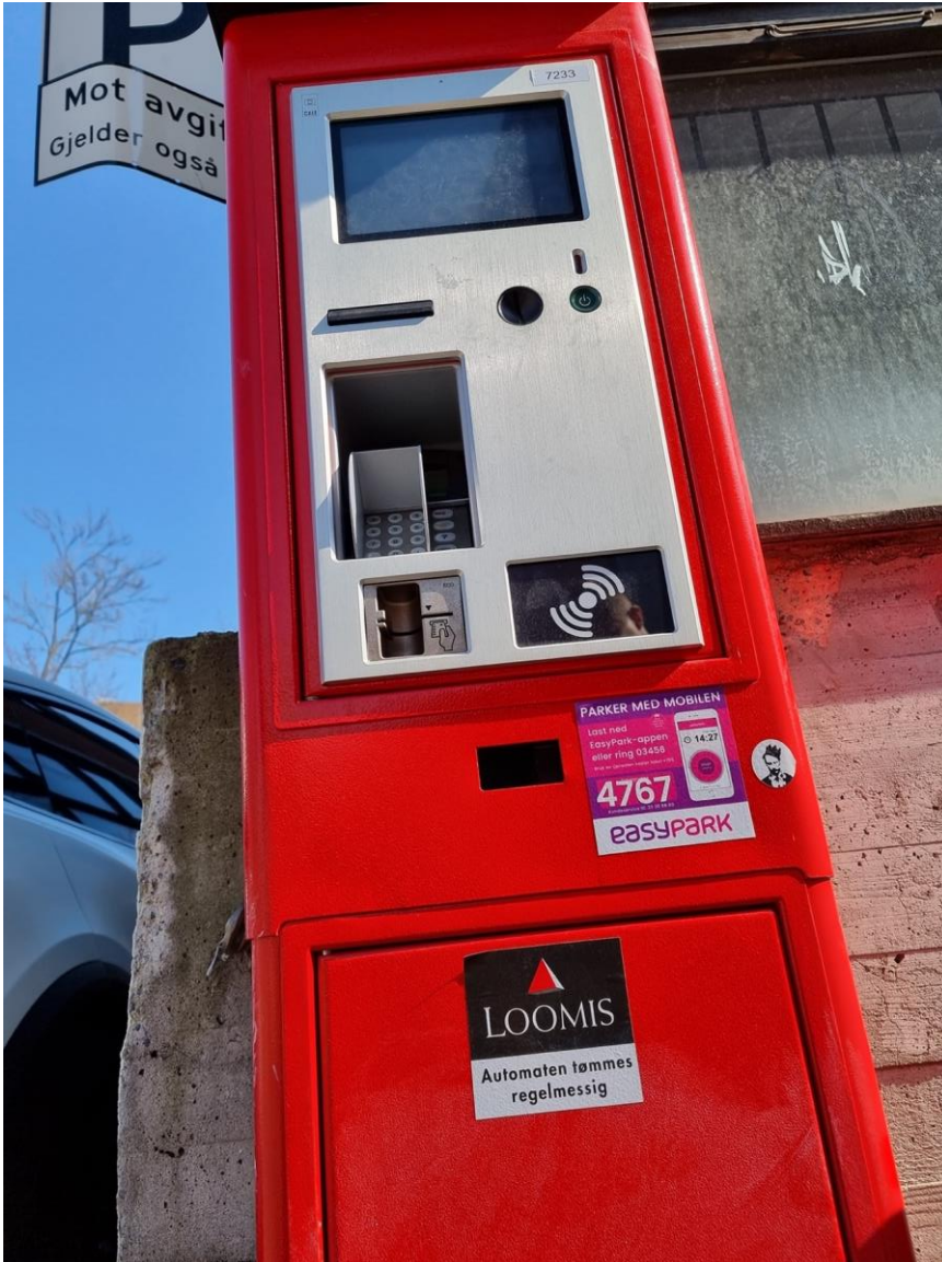
Figure 11 Parking ticket machine, picture taken from a lower position, there is no perceptible information on the display
