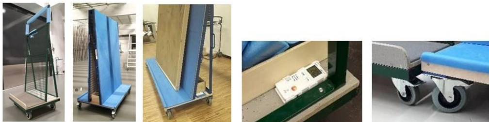
Fig. 1. From left: Small trolley, small wheels, without foam. Large trolley with foam, angle twin unit walls, large wheels, Ø12, 2 cm thick rubber part. Small trolley with foam, single unit wall, large wheels, Ø12, 2 cm thick rubber part. Testo placed in corner on the width. Testo placed in the corner at the long side on small trolley. Small and large wheels.
