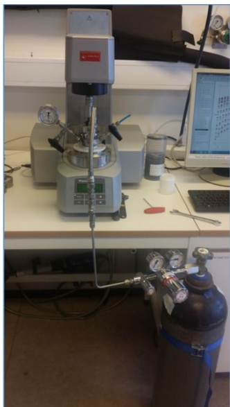
(a) Anton Paar MCR 301 Rheometer with the connected nitrogen tank used for running the experiment
