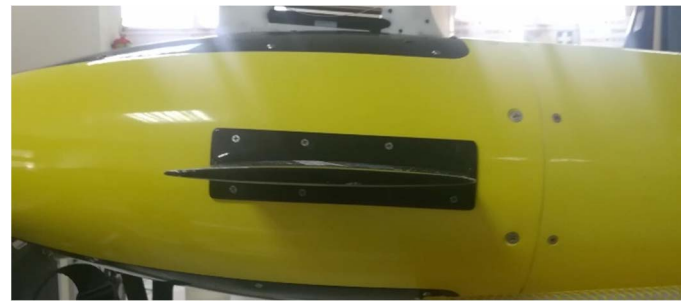
Fig. 6. Seaglider wings cross-sections (image by the author)
