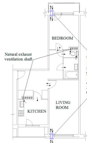
Figure 13: Principle of placement of Pair-Wise DV, plan view (Mikola et al., 2019)
