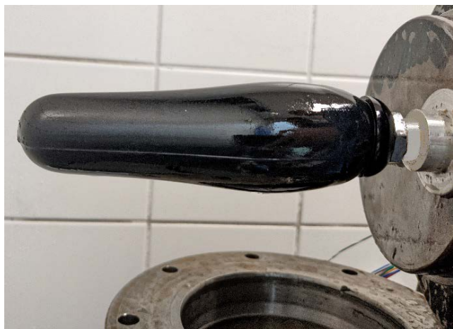
FIGURE 7. Oil bladder directly after testing in the pressure vessel.
