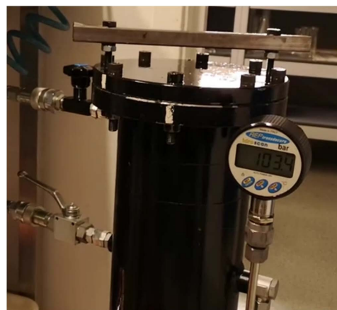
FIGURE 9. Pressure testing rig with digital pressure gauge, that is used to perform VBS tests.
